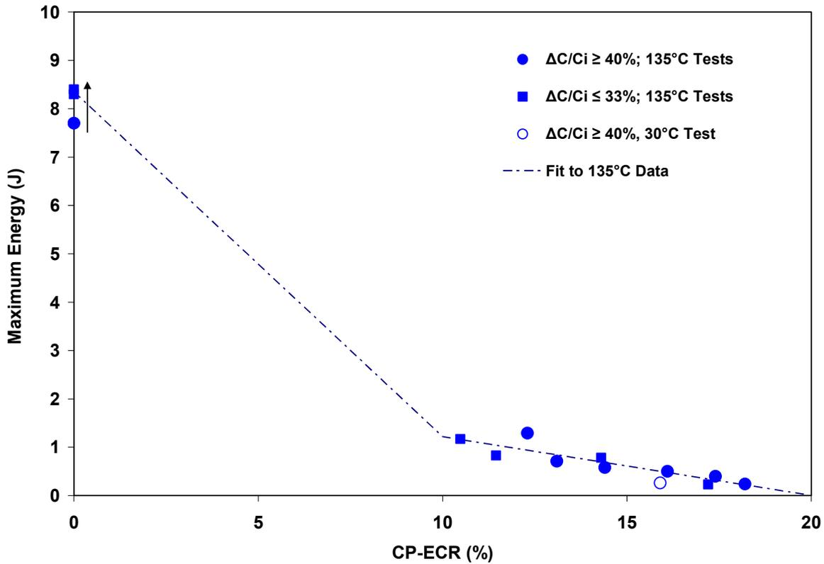
**Figure 4** Maximum (for 0% CP-ECR) and failure (for  $\geq 10\%$  CP-ECR) energy as a function of oxidation level (CP-ECR) for post-LOCA samples subjected to four-point bending with the rupture region in tension for all tests but one. Bend tests were performed at 135 °C and 2 or 1 mm/s to 14-mm maximum displacement. One bend test was conducted at 30 °C and 1 mm/s.
