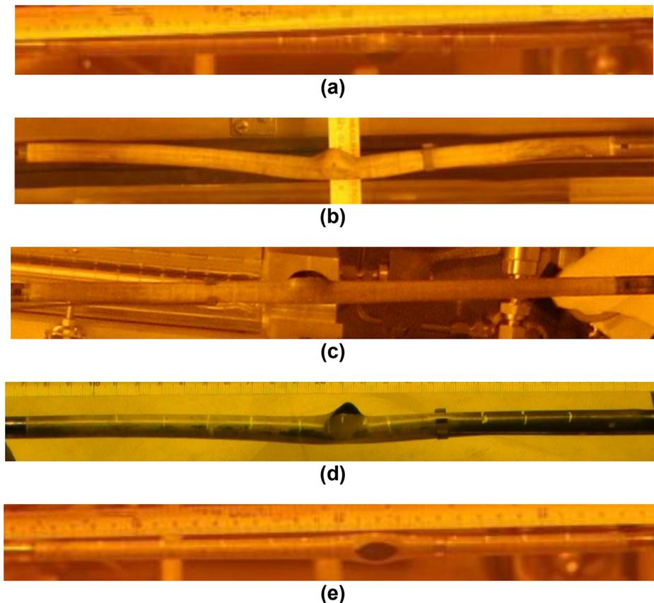
**Figure 16** Image of rod segment showing any distortion out of plane, with the rupture from (a) Test 189, (b) Test 191, (c) Test 192, and (d) Test 193. (e) is an image of rod segment 189 taking in-plane of the rupture, showing no significant rod bending that is characteristics of all other tests.
