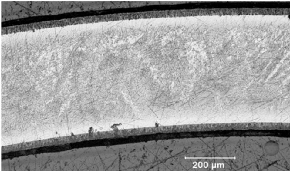
(b) Back side of rupture node cross section
