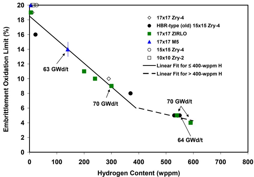
**Figure 1 Embrittlement oxidation limit (CP-ECR in %) as a function of metal hydrogen content for as-fabricated, prehydrided, and high-burnup cladding alloys oxidized at a peak temperature of 1,200 °C, quenched at 800 °C, and ring-compressed at 135 °C. Oxidation values above data points and trend lines resulted in brittle behavior. For hydrogen contents in the range of 540–600 wppm, peak cladding temperatures (1,130–1,180 °C) occurred during the heating ramp at <1,200 °C (Ref. 6).**
