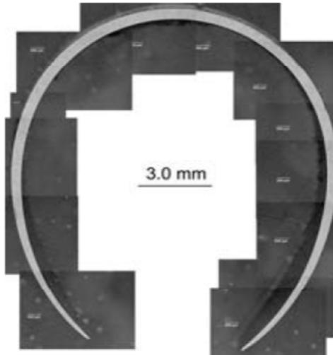
**Figure 2 Ballooned and ruptured ZIRLO cladding (ANL)**
