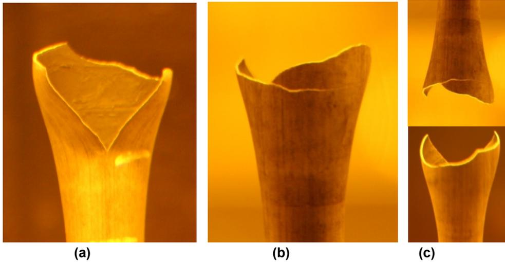
**Figure 22** Images of the fracture profile from segment 191 after the four-point bend test: (a) the bottom half, (b) the top half, and (c) an illustration of the back side of the two halves put together. In (b) a second crack propagation path can be seen.
