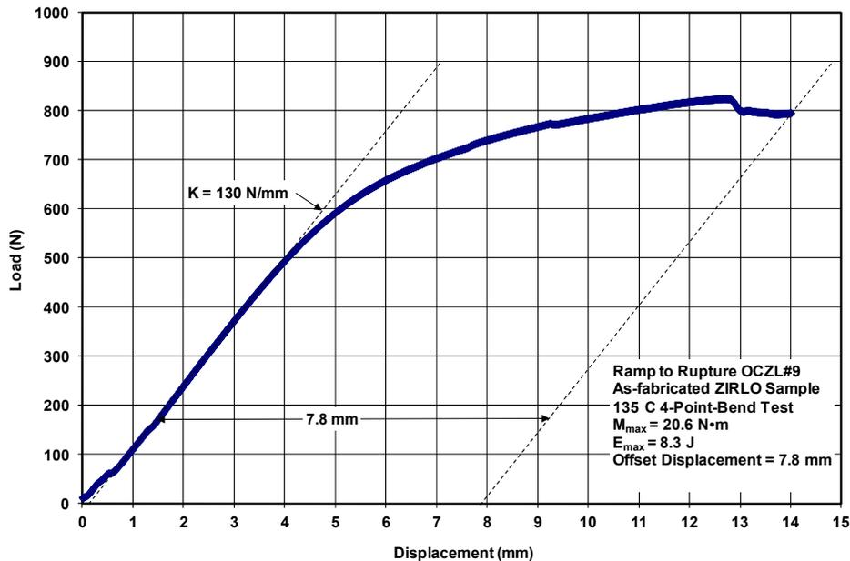
**Figure 5 Four-point bend test load-displacement curve for ramp-to-rupture sample OCZL#9. The as-fabricated ZIRLO sample ruptured at  $875\pm 15$  °C with a mid-wall rupture strain of 33%. The 4-PBT was conducted at 135 °C and 2 mm/s displacement rate to 14-mm maximum displacement.**
