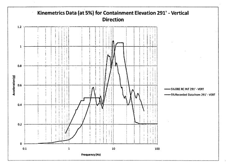
The figure above, as submitted by the licensee, compares the observed ground motion in the vertical direction to the exceeded design motion at various frequencies. The blue curve is from the observed readings and the purple curve is the design spectrum at the same elevation level.
