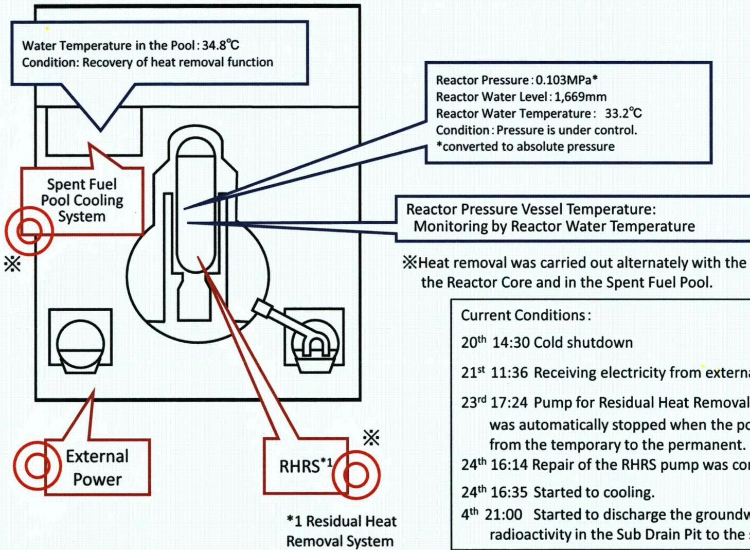
※Heat removal was carried out alternately with the water in the Reactor Core and in the Spent Fuel Pool.
