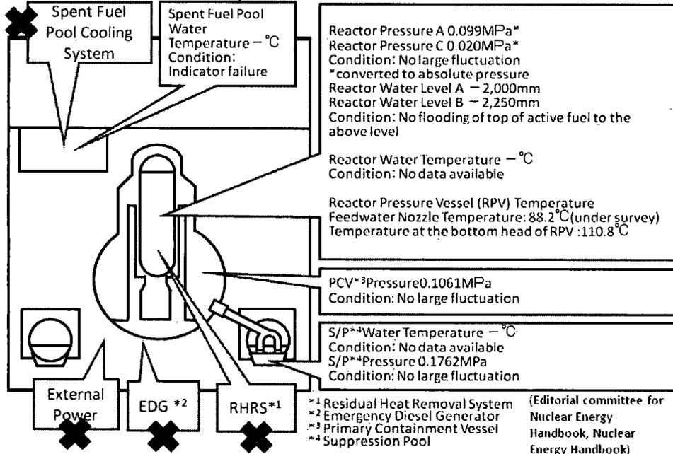
**Unit 4 No fuel is in the reactor pressure vessel. Fresh water is being injected to the spent fuel pool.**
