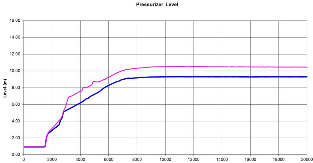
**Figure 20: F2.2 Run 1 and Run2 pressurizer level calculation**
