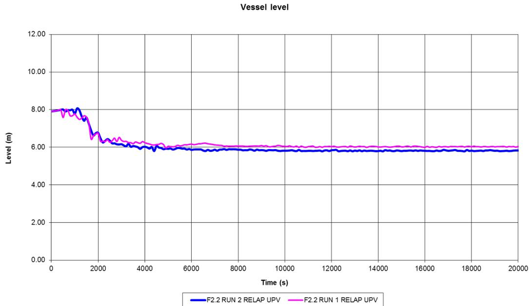
**Figure 21: F2.2 Run1 and Run2 vessel level calculation**
