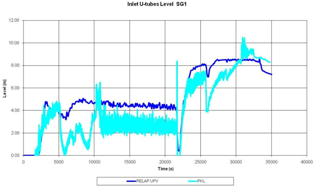
**Figure 6: Water level inlet side of SG1 U-tubes**
