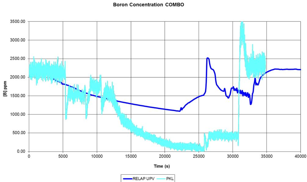
**Figure 10: Boron concentration in loop seal one**
