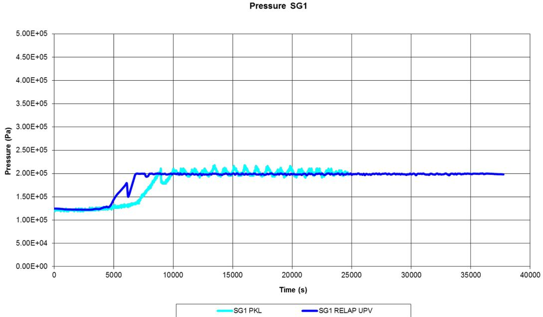
**Figure 13: Pressure in the SG1 Secondary Side**
