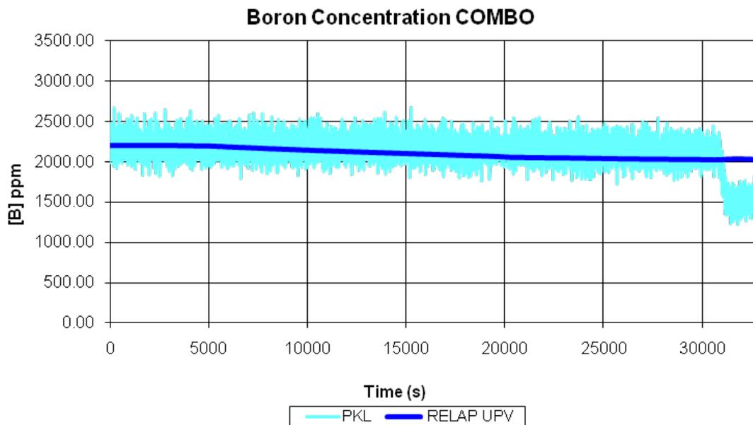
**Figure 18: Boron concentration at the core inlet**
