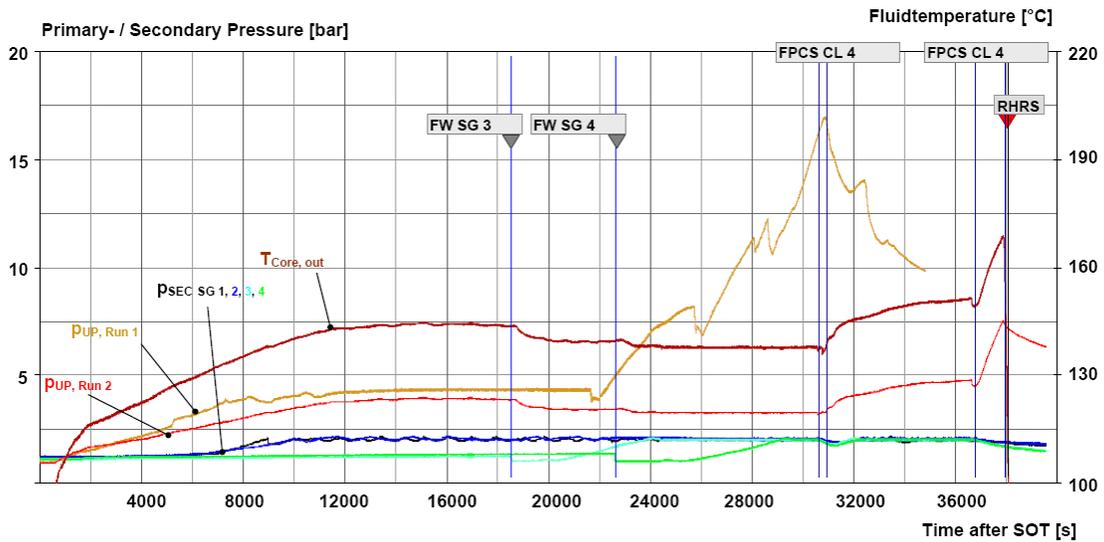
**Figure 3: Primary and Secondary Pressure in F2.2 Run 2**
