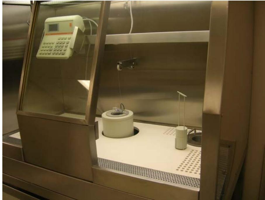
Dispensing station with dose calibrator
