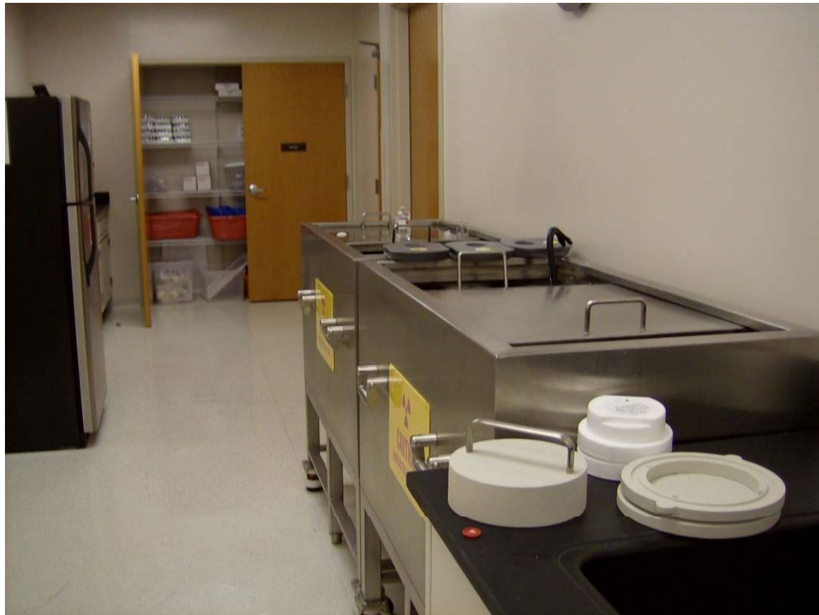
Shielded boxes for generators (coffins)
