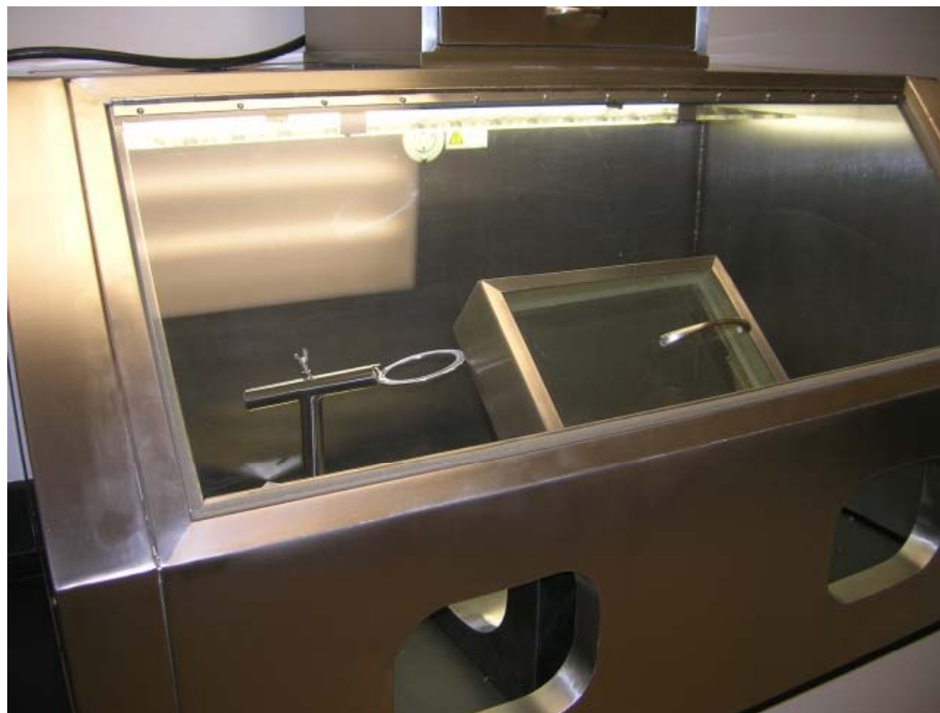
Glove box for preparing iodine capsules
