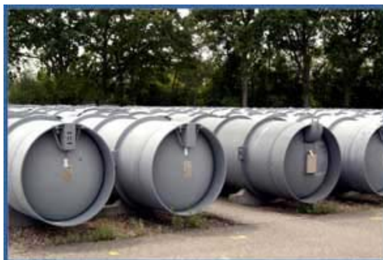
Figure 7-6. Urenco DU UBCs (Note: thick walled 48Y Cylinders, not 48G Cylinders as used at DOE and USEC facilities in the U.S.)
