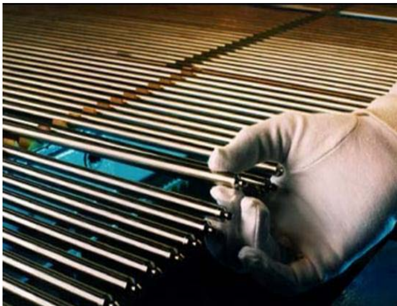
Figure 5-15. Visual Inspection of Rod Ends
