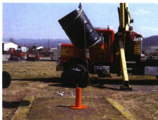
HAC 1 Meter Center of Gravity Puncture Drop Height Position
