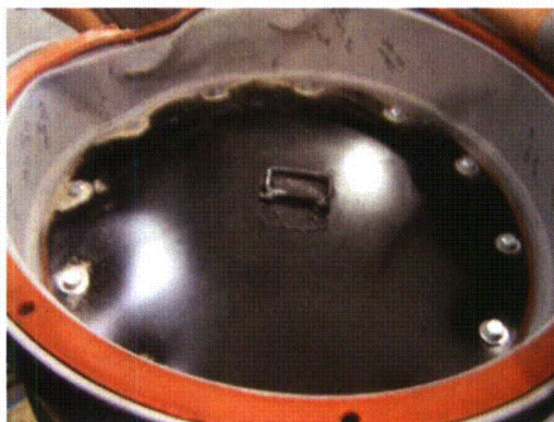
Bulge in Containment Blind Flange Showing Loose Sand from Containment Cavity
