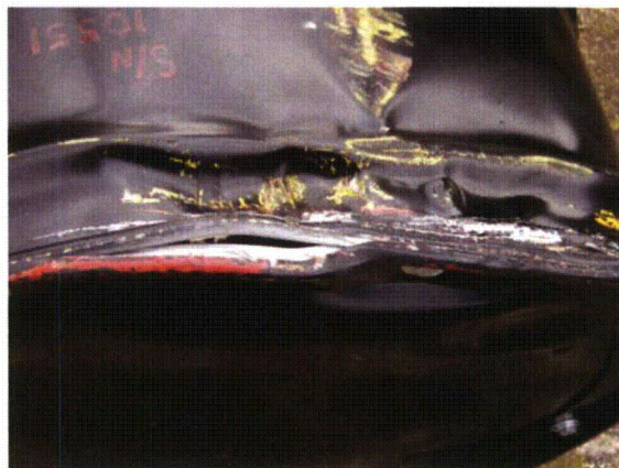
Close-up Top End Damage 1/4" x 1-1/14" Gap – Metal to Metal Seal No Opening
