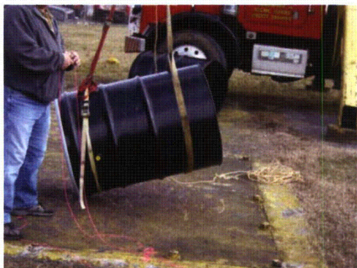
Shallow Angle Accelerated Drop Set-up 17° Angle of HAC Shallow Angle Drop
