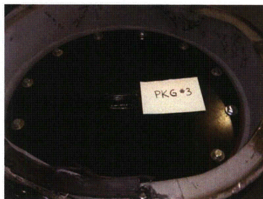
½" Thick Inner Blind Flange Post Test Flat & No Loss of Payload Contents
