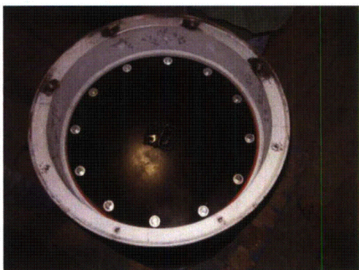
Top View of 1/2" Thick Blind Flange
