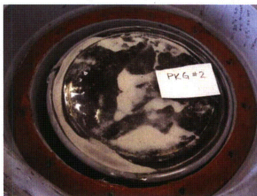
Payload and Lose Sand Remained within the Containment Cavity
