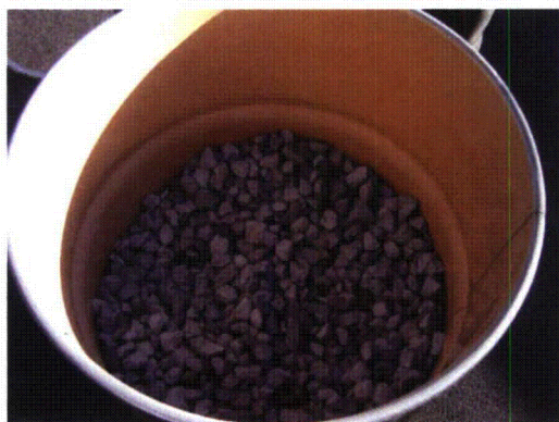
30 Gallon Drum Loaded With 260 Pounds of Loose Gravel
