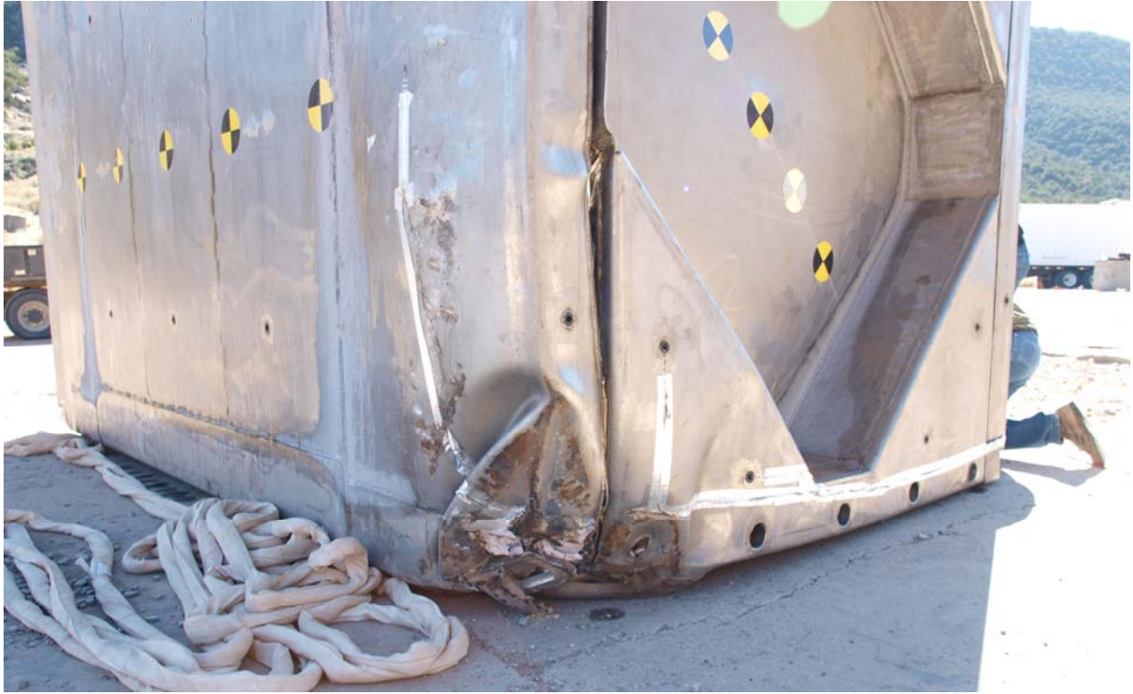
Figure 2.12.6-11 – Test LD91, CG-Over-Corner Free Drop Damage
