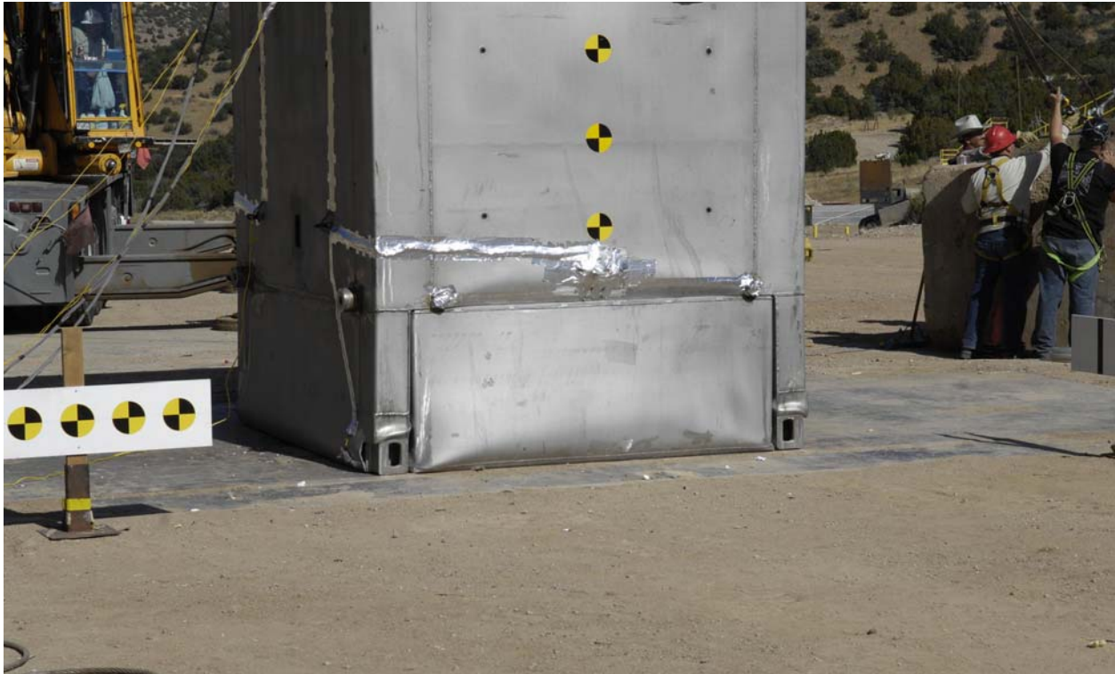
Figure 2.12.3-10 – Test LD2, Typical Deformations at Closure End
