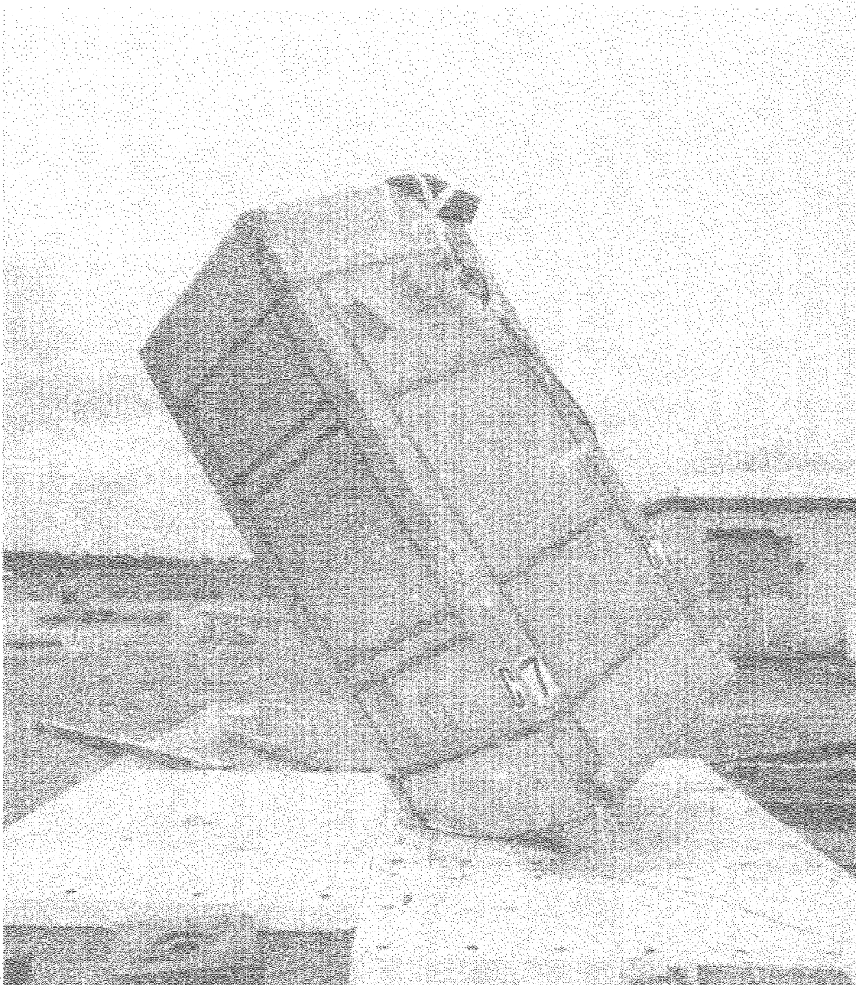
Figure 2.12.1-22 – Free Drop Test C7: View Immediately Following Impact
