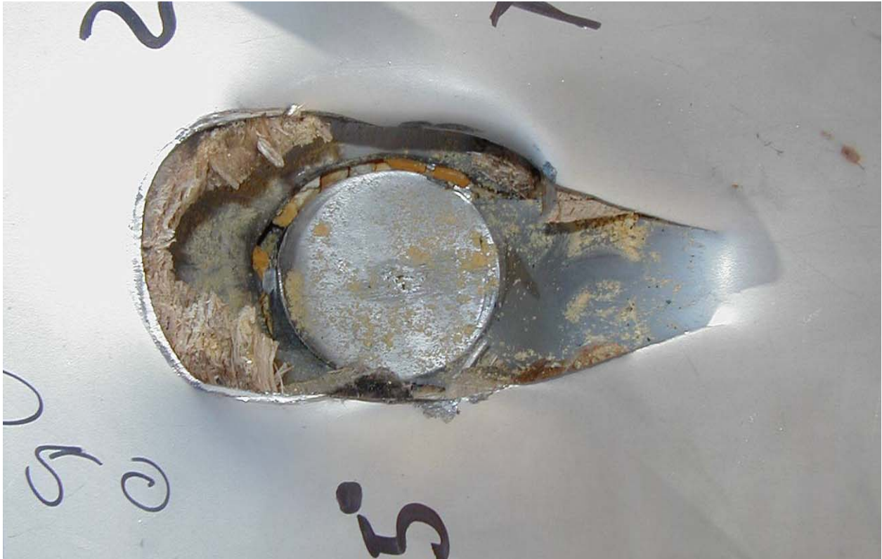
Figure 2.12.1-59 – Puncture Drop Test P305 at 25°
