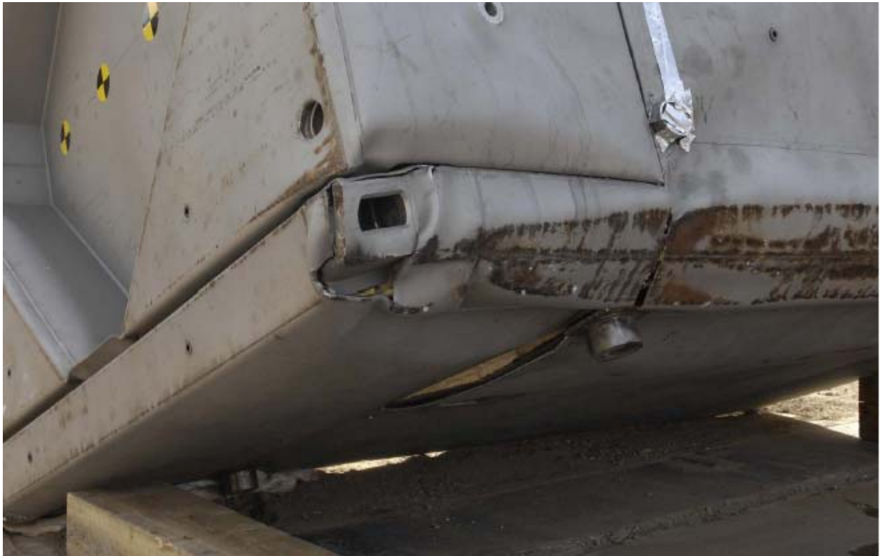
Figure 3.5-20 – Weld Tear from LD-5 Free Drop Orientation
