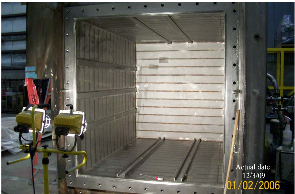
Figure 2.12.6-20 – Payload Cavity with All Contents Removed
