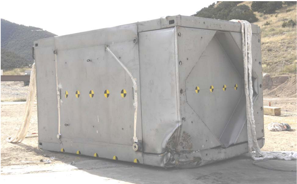
Figure 2.12.3-19 – Test LD4, Typical Deformations
