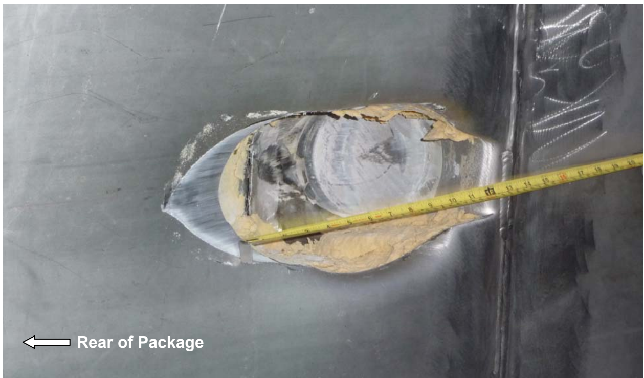
Figure 2.12.6-14 – Test LP92, Puncture on Bottom Wall Damage
