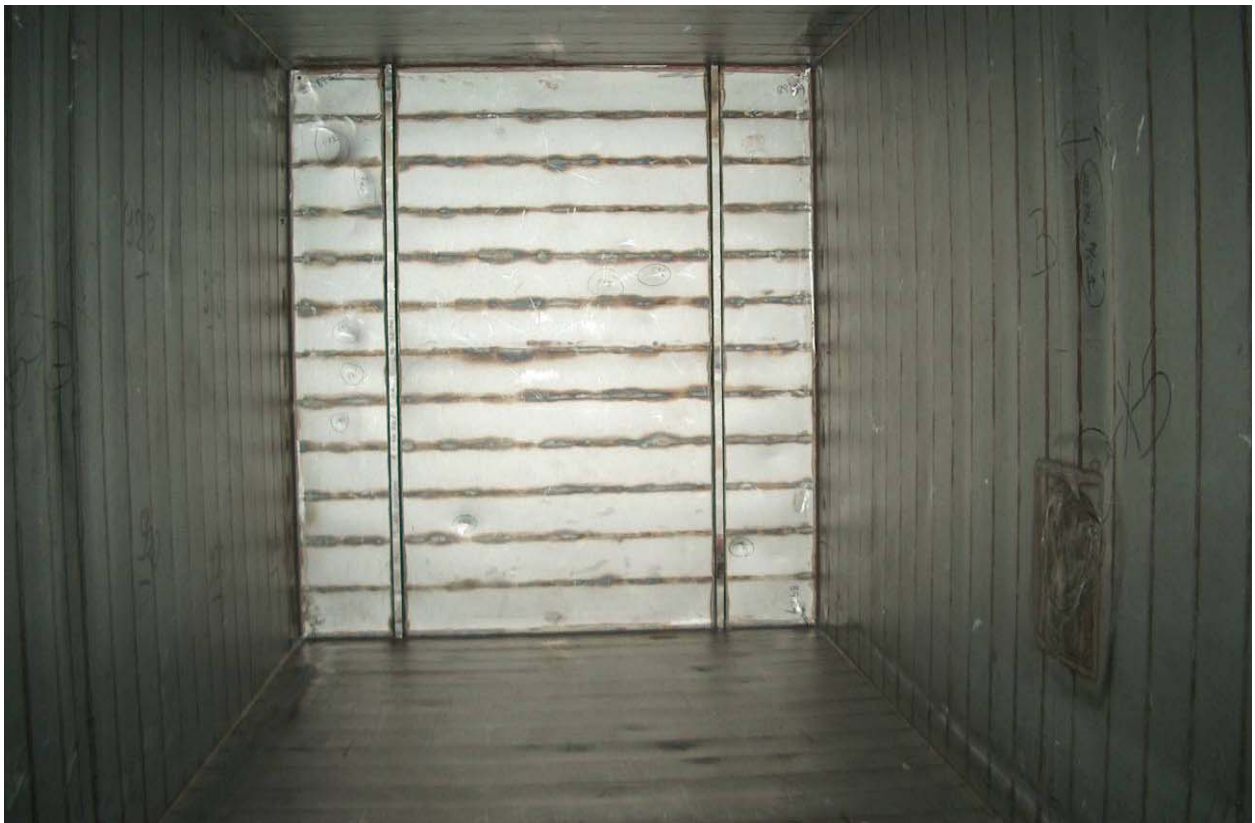
Figure 2.12.1-54 – Post-Test Disassembly: View of Cavity with Payload Removed
