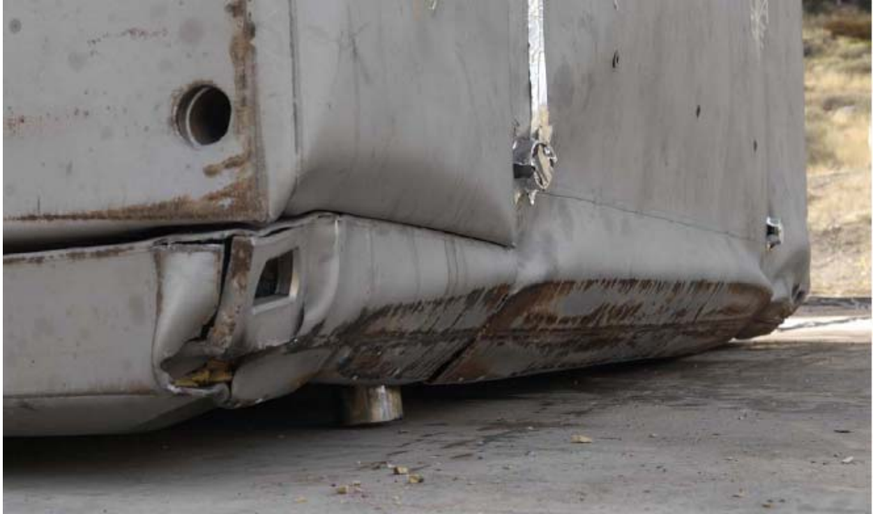
Figure 3.5-19 – Edge Deformation from LD-5 Free Drop Orientation
