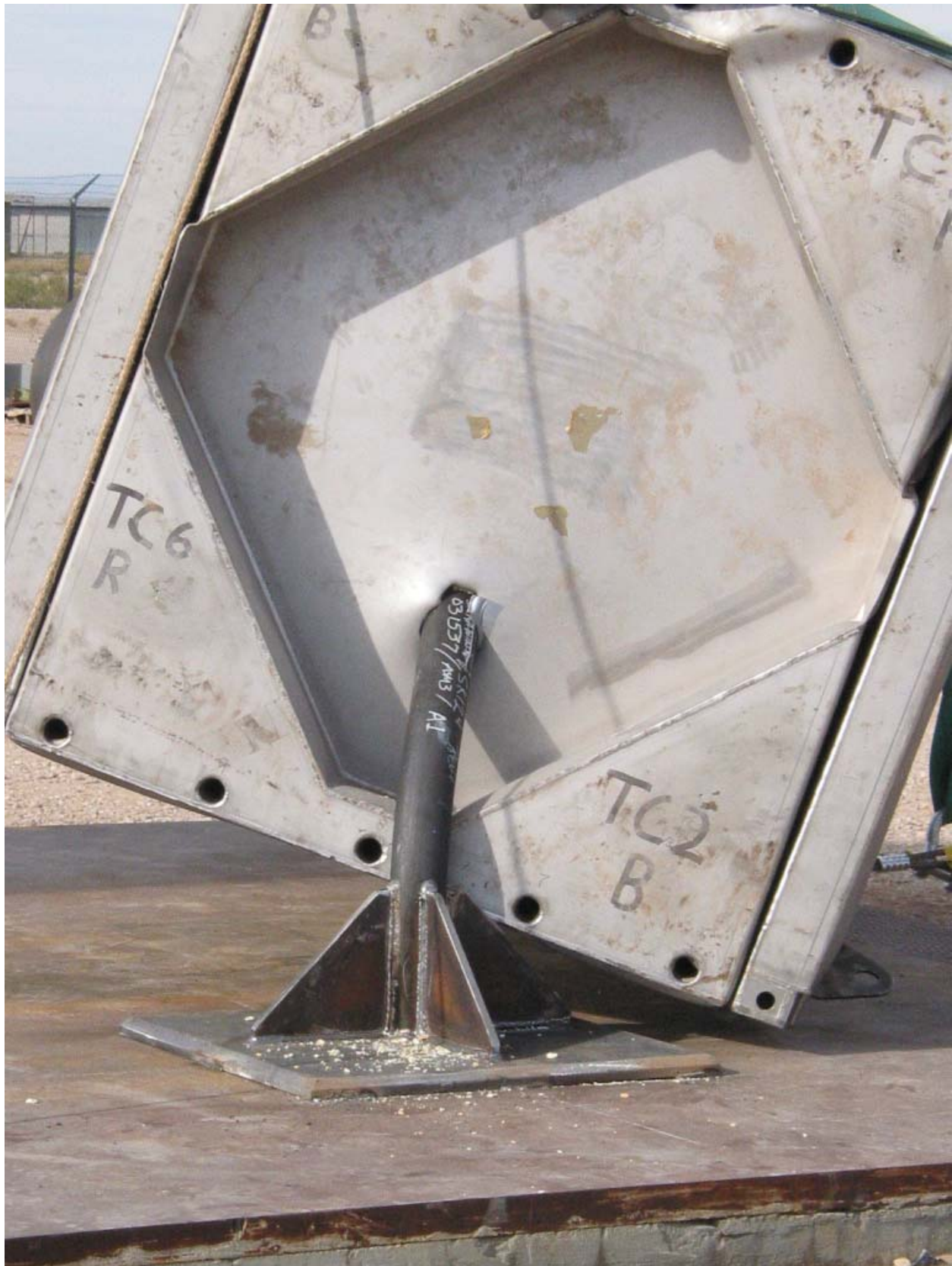
Figure 2.12.1-43 – Puncture Drop Test P1: Overall View Immediately After Impact
