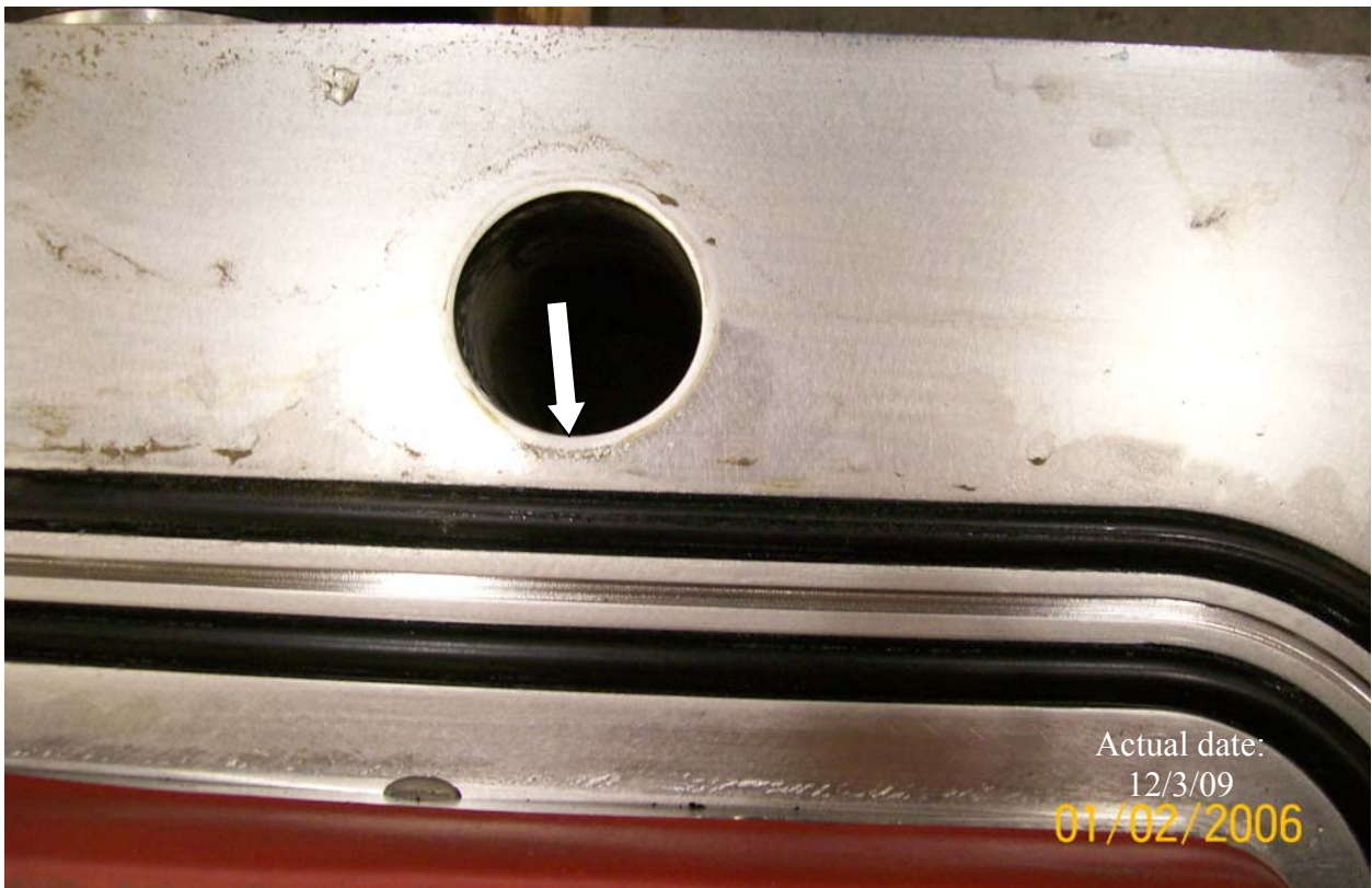
Figure 2.12.6-18 – Galling on Flange Around Closure Bolt Holes
