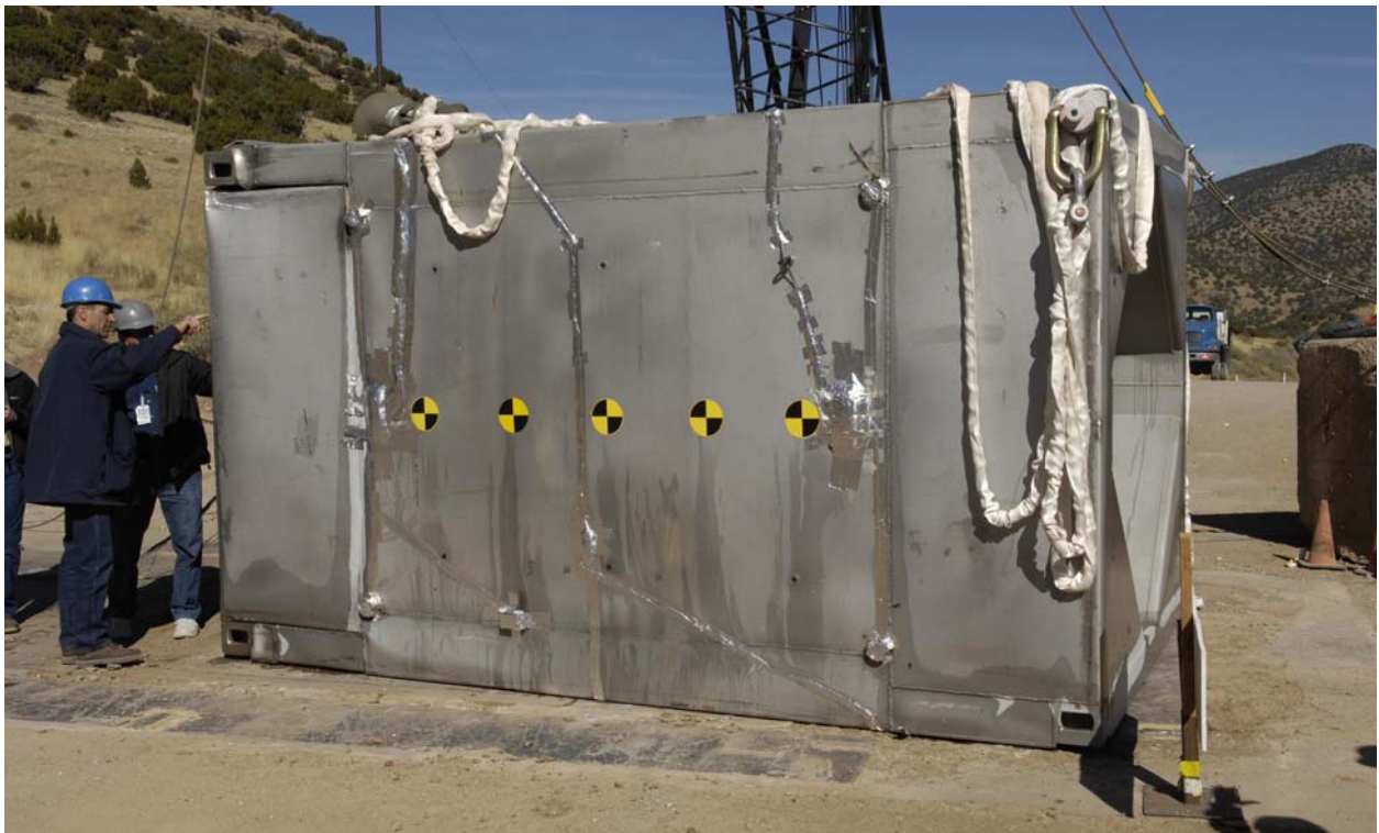
Figure 2.12.3-13 – Test LD3, Typical Side Deformations (Impact Side Down)
