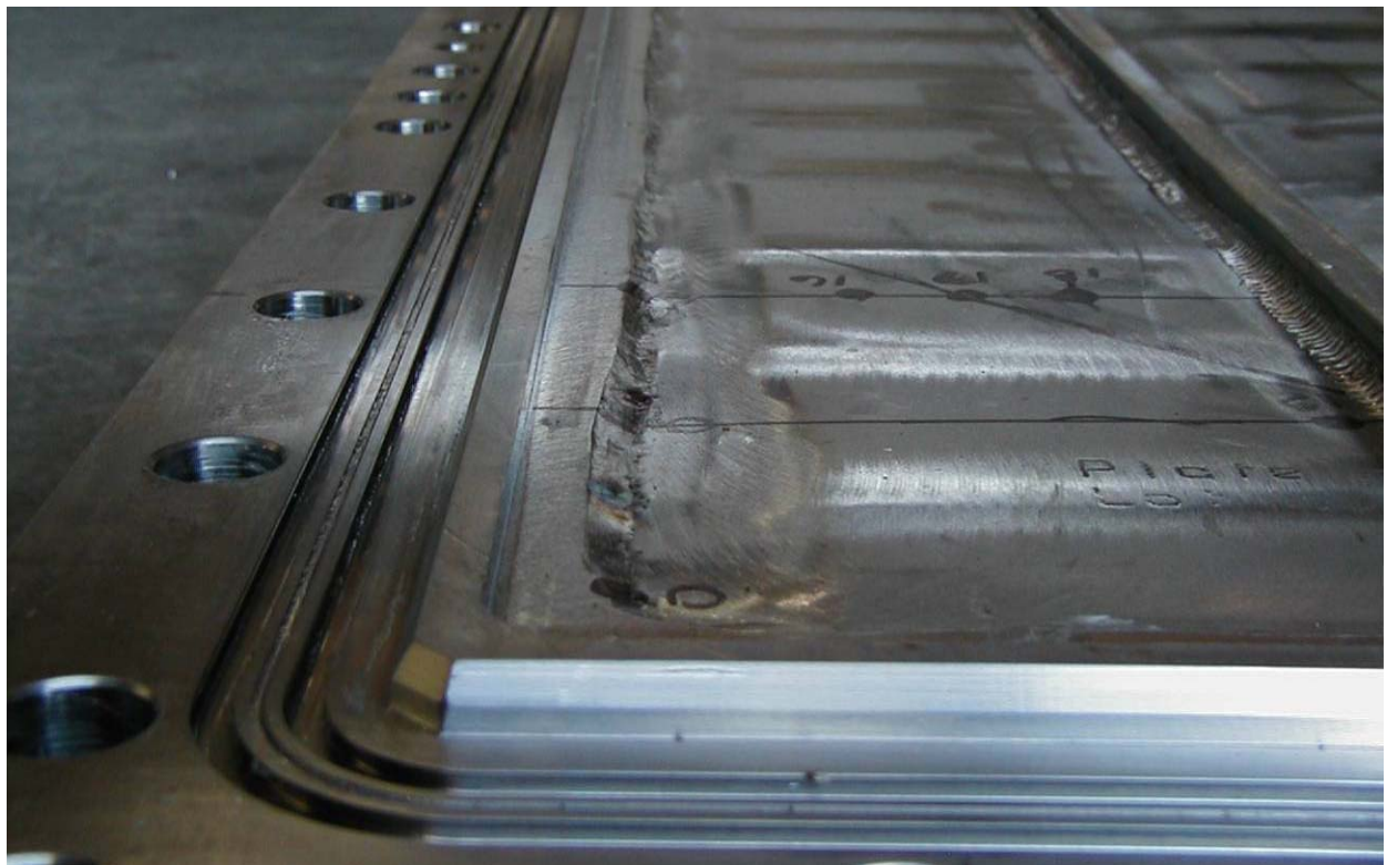
Figure 2.12.1-56 – Post-Test Disassembly: Close-up View Closure Lid O-ring Seal Grooves
