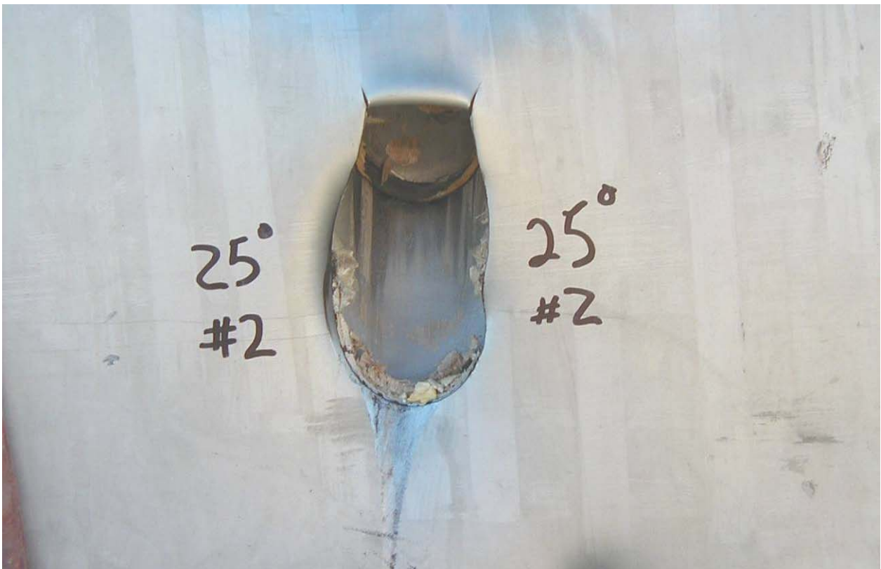
Figure 2.12.1-60 – Puncture Drop Test P405 at 25°
