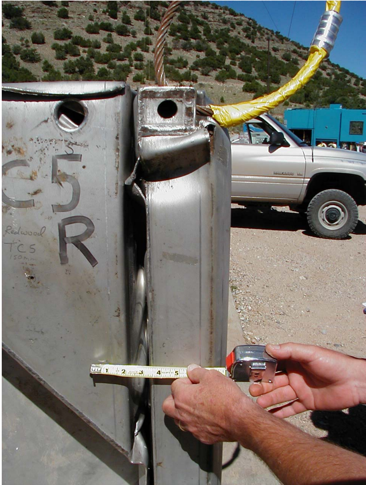
Figure 2.12.1-40 – Free Drop Test FD4: Close-up View of Secondary Impact Damage
