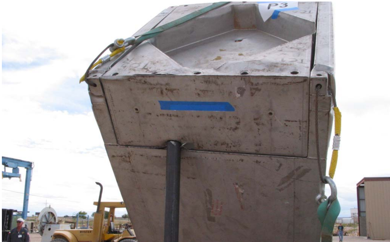
Figure 2.12.1-47 – Puncture Drop Test P3: Overall View Immediately After Impact
