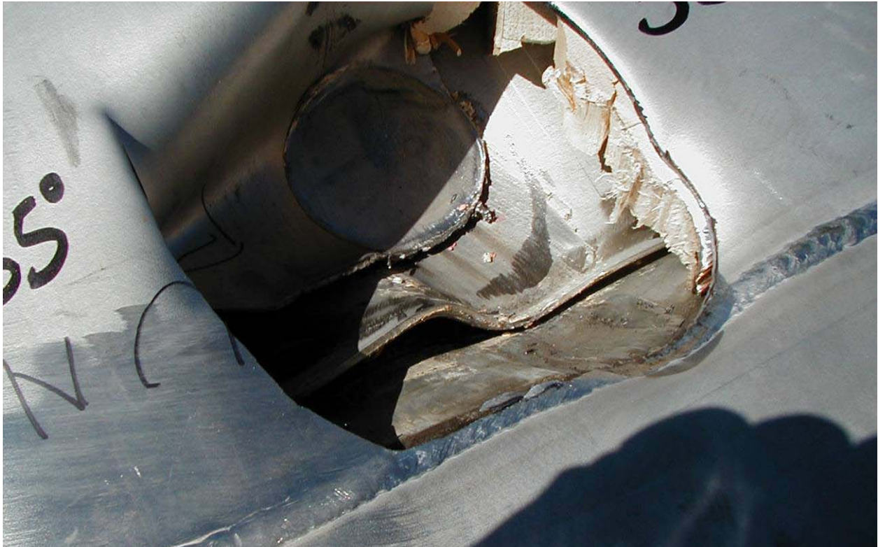
Figure 2.12.1-57 – Puncture Drop Test P105 at 35°
