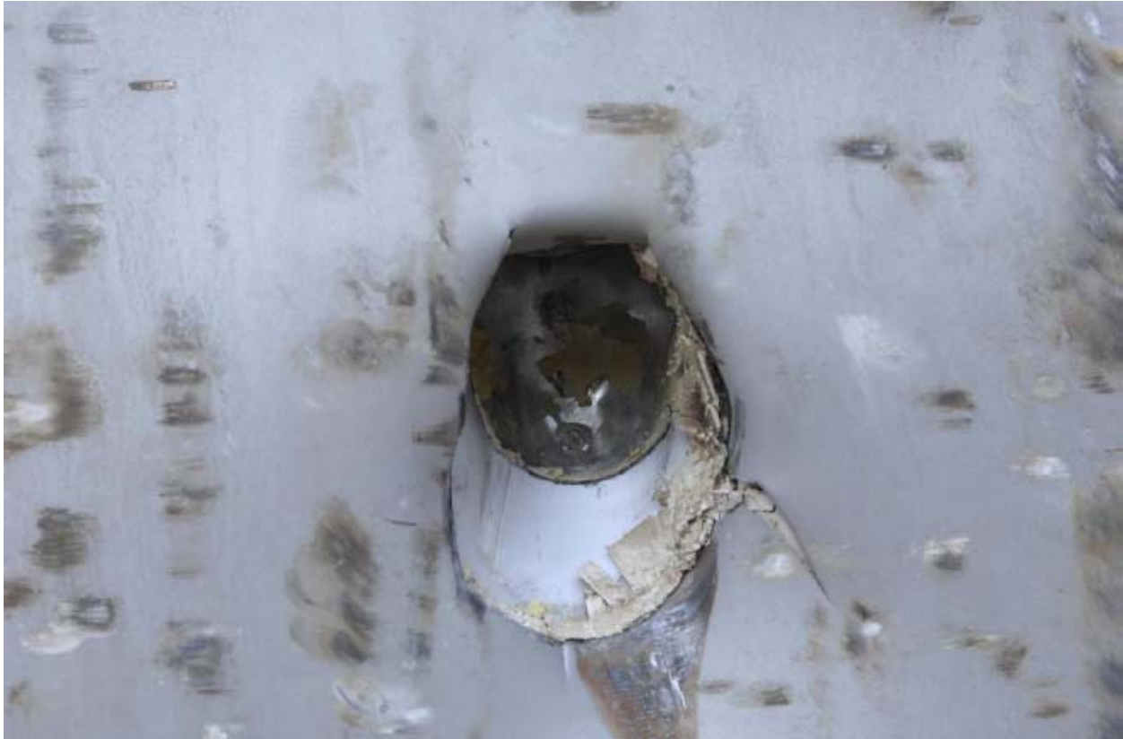
Figure 3.5-23 – LP1 Puncture Bar Damage after Removal of Bar
