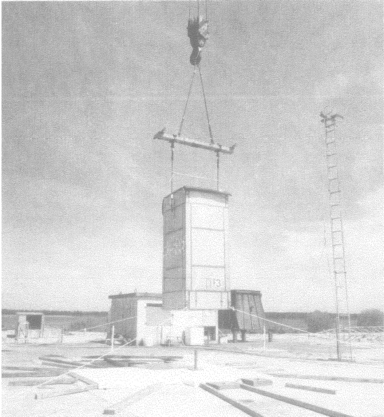
Figure 2.12.1-12 – Puncture Drop Test F3: Pre-Test View of CTU Orientation
