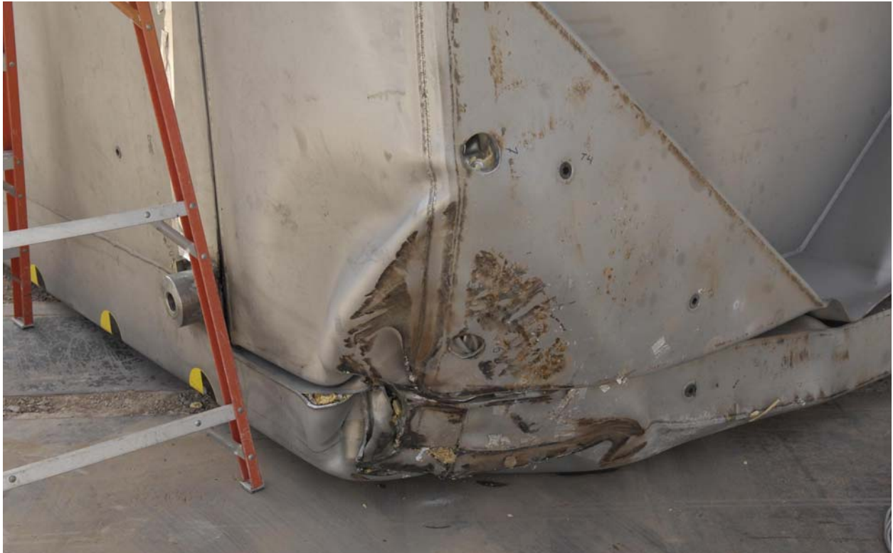
Figure 2.12.3-20 – Test LD4, Close-up of Deformations
