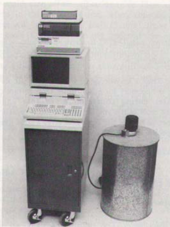
Figure 1. - Controlling and recording instrumentation for conducting tests to determine specific heat of concrete.
