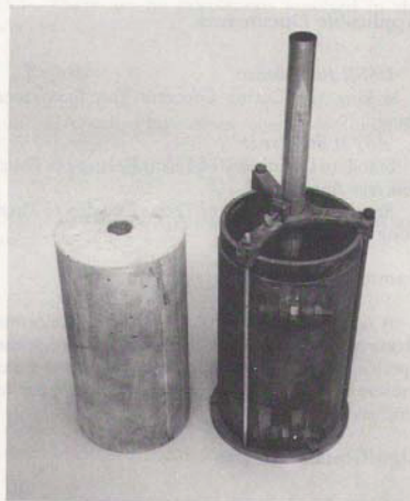
Figure 3. - Mold and 8- by 16-inch (203- by 406-mm) cylinder with a 1.5-inch (38-mm) hole through the center.
