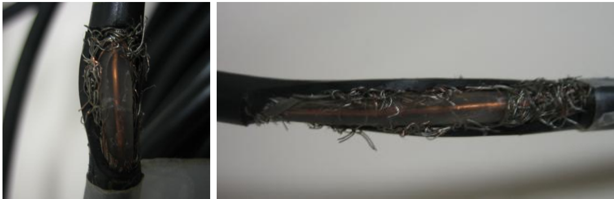
Figure 6. RG-58 cable with 1-3 cm sections of outer jacket removed around half of the cable circumference.
