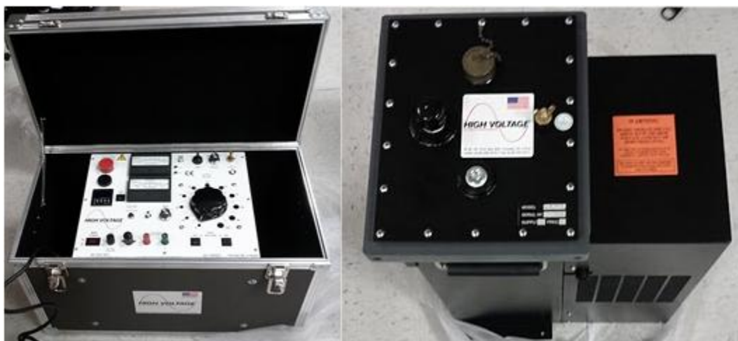
Figure 3. Newly acquired test equipment: Controller for Very Low Frequency (VLF) source, LC meter, and instrumentation (left) and VLF High Potential Test Source up to 65kV (right).
