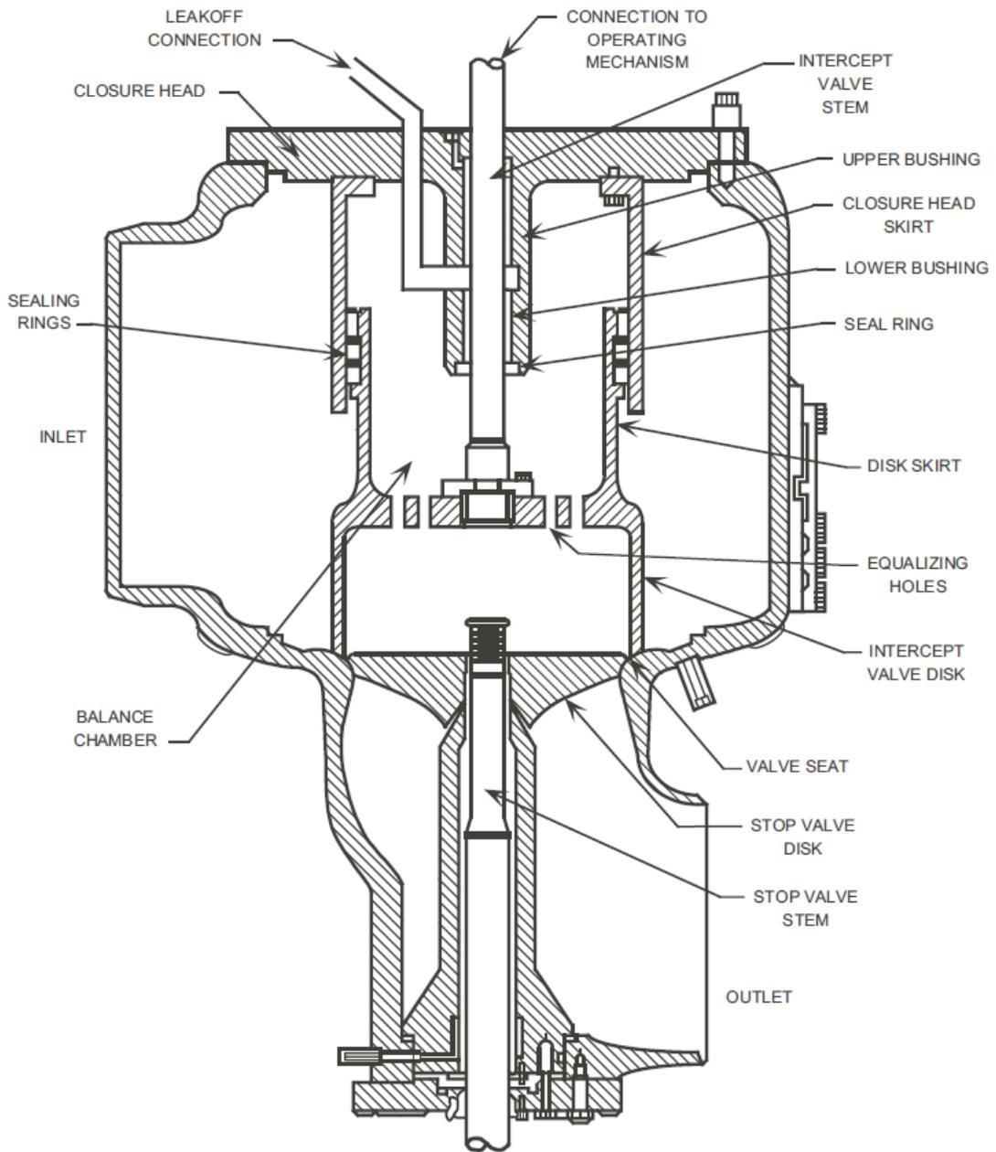
Figure 7.4-5 Combined Intermediate Valve
