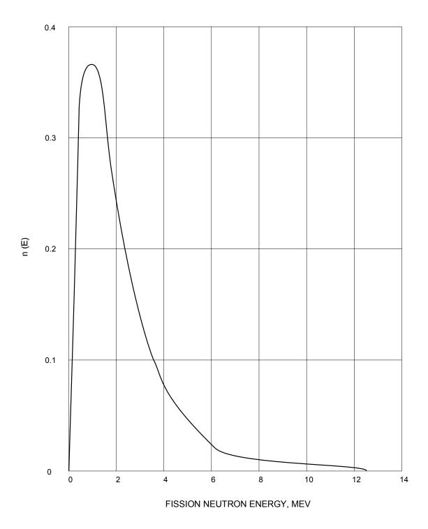
Figure 2.1-1 Fission Neutron Energy
