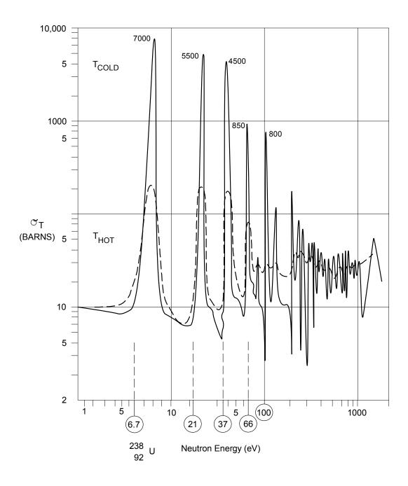
Figure 2.1-4 Cross Section Curve
