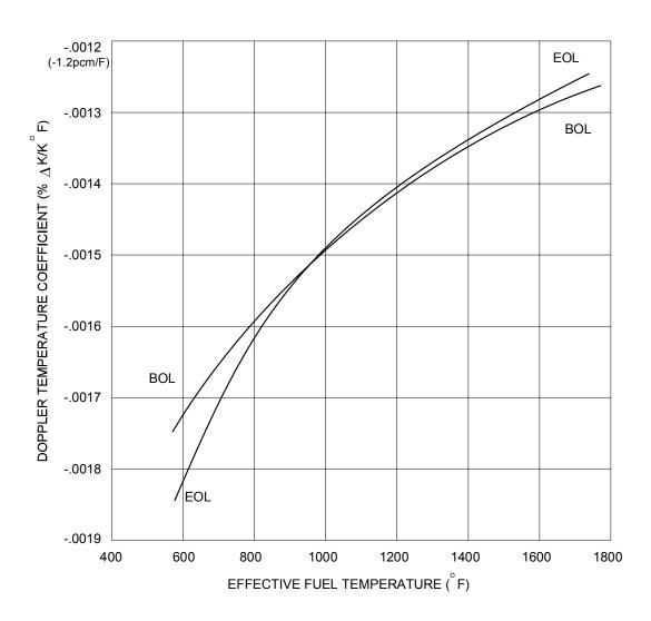
Figure 2.1-5 Doppler Temperature Coefficient, BOL and EOL
