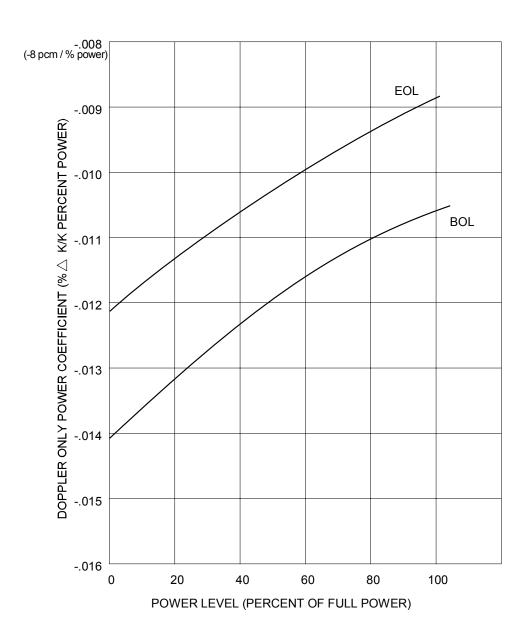
Figure 2.1-6 Doppler Only Power Coefficient, BOL and EOL
