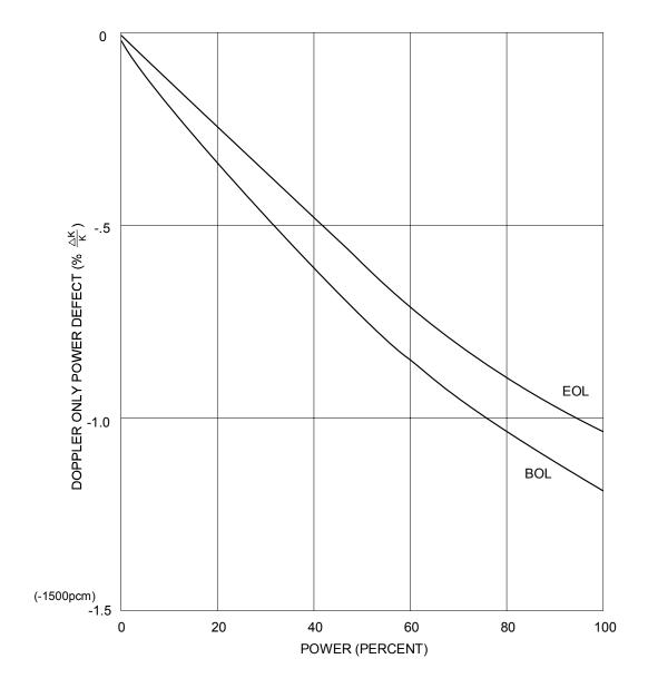
Figure 2.1-7 Doppler Only Power Defect, BOL and EOL
