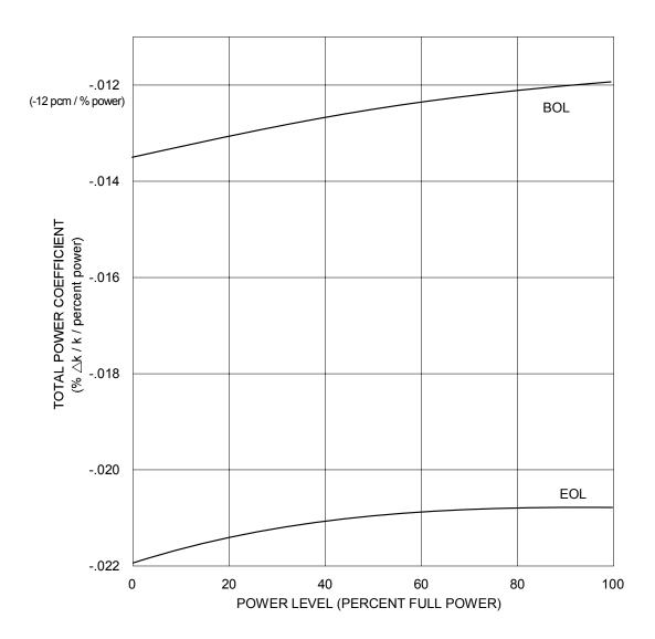
Figure 2.1-9 Total Power Coefficient, BOL and EOL
