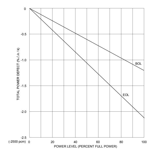
Figure 2.1-10 Total Power Defect, BOL and EOL
