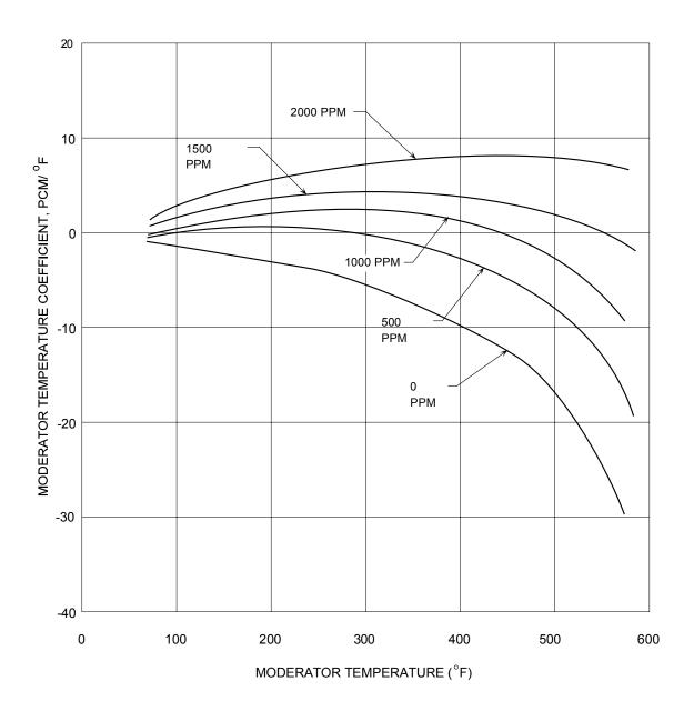
Figure 2.1-8 Moderator Temperature Coefficient
