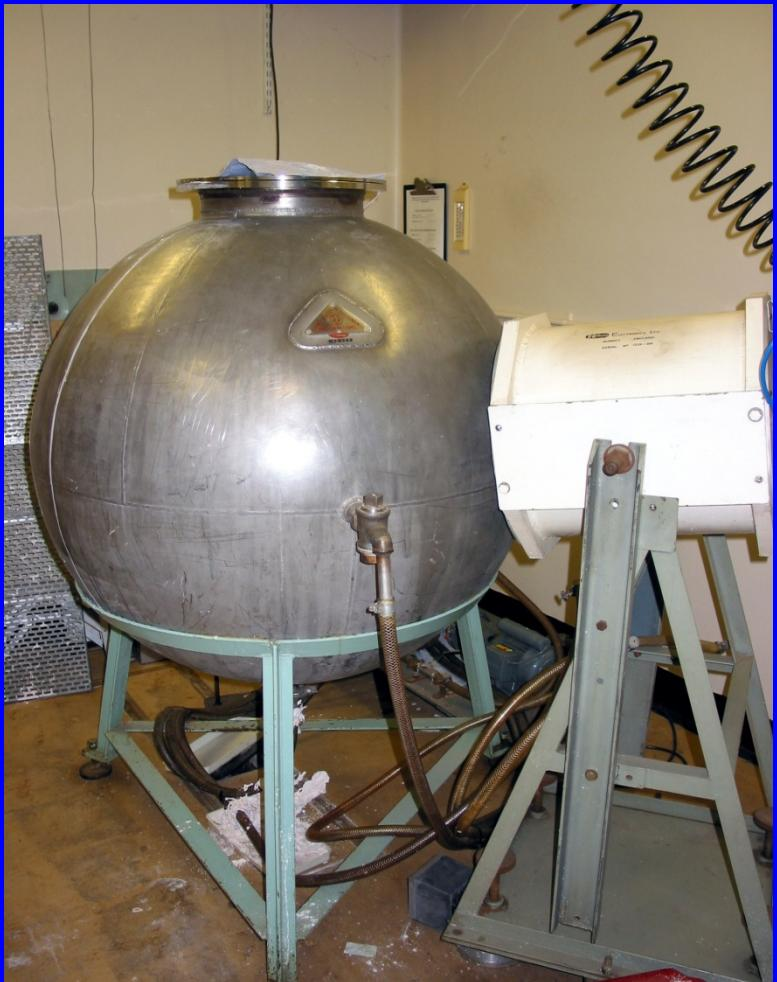
The manganese solution is inside the spherical tank and the source is lowered through the top.
