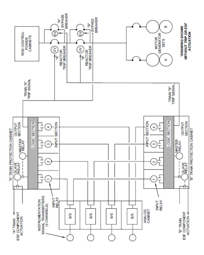
Figure 12.1-2 Solid State Protection System
