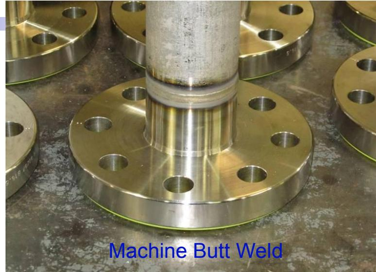
Machine Butt Weld
