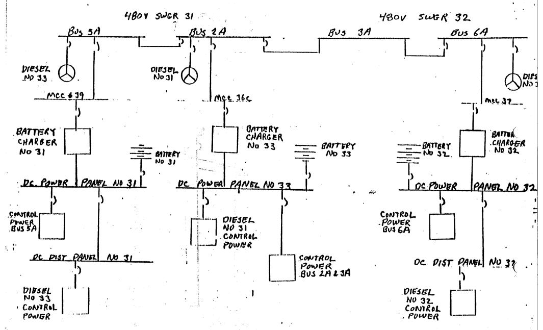
SIMPLIFIED DIAGRAM OF MOIAN POINT UNIT 2 120 VOLT AC INSTRUMENT DISTRIBUTION SISTES
