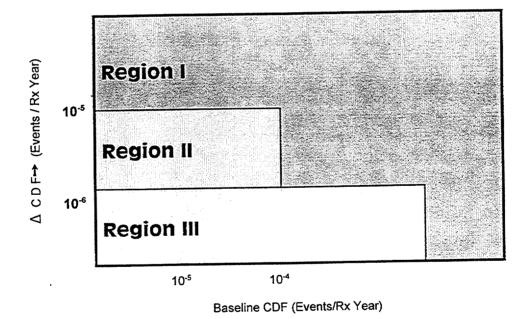
Figure 2.1 Acceptance Guidelines for Core Damage Frequency (CDF) (Adapted from Figure 3 of RG 1.174)
