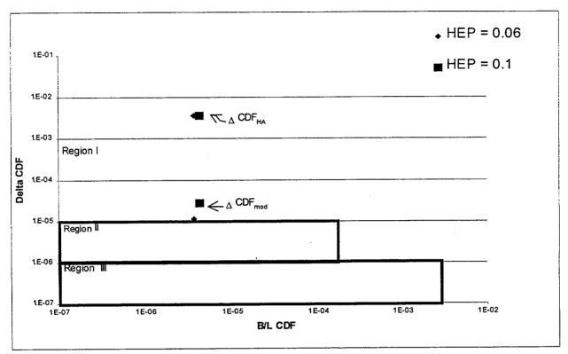
Risk screening calculations for Step 1 for  $\Delta \text{CDF}_{mod}$  were conducted and the results plotted in Figure B.3.
