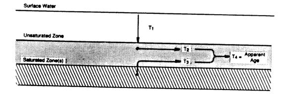
Figure 1. Apparent age of a groundwater (T4) may result from mixing of several groundwaters of differing ages and processes.
