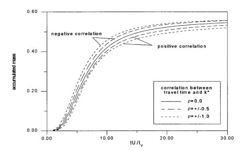
Figure 5-3. Effect of correlation between  $k^*$  and  $\tau$  on the cumulative breakthroughs. The following moments are used in the lognormal distribution:
