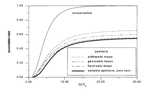
Figure 5-4. Comparison between different effective (mean) values of  $k^*$  and a case with variable  $k^*$  (zero correlation).
