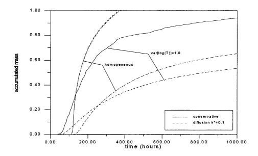
Figure 4-5. Comparison between conservative and diffusion affected cumulative breakthroughs for homogeneous and heterogeneous flow conditions.
