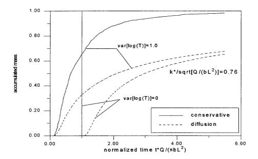
Figure 5-2. Comparison between conservative and diffusion affected cumulative breakthroughs for homogeneous and heterogeneous flow conditions.
