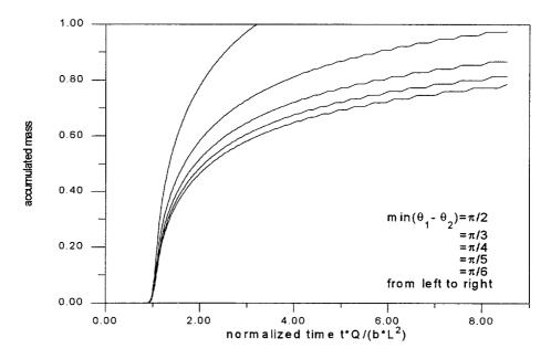
Figure 4-2. Effect of streamline configuration on the cumulative breakthrough of mass in the abstraction borehole.
