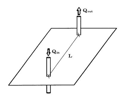
Figure 4-1. Experimental set-up for the MWTE with two boreholes separated by a distance L injecting and abstracting water at a flow rate Q.
