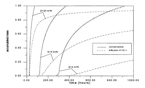
Figure 4-4. Effect of pumping rate on the cumulative breakthrough.
