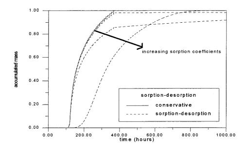
Figure 4-8. Effect of increasing sorption coefficients on the cumulative breakthrough.
