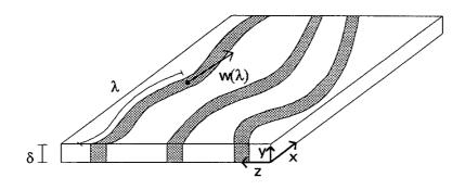
Figure 2-1. Fracture plane with aperture  $\delta$ . The velocity at a distance  $\lambda$  along the first streamline is w.
