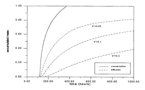
Figure 4-3. Influence of the magnitude of the  $k^*$ -value on the cumulative breakthrough.
