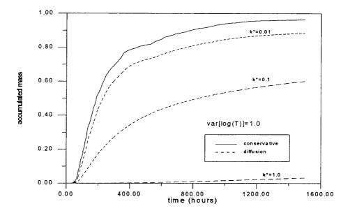
Figure 4-6. Effect of a tenfold increase or decrease in the diffusion parameter  $k^*$  on the cumulative breakthrough.
