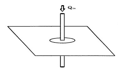
Figure 5-1. Experimental set-up for the MDE with one centrally located injection borehole. The control surface is indicated around the borehole.
