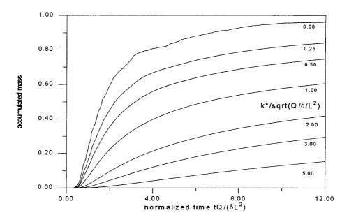
*Figure 4-7.* Dimensionless nomogram presentation of the results for the given transmissivity statistics.
