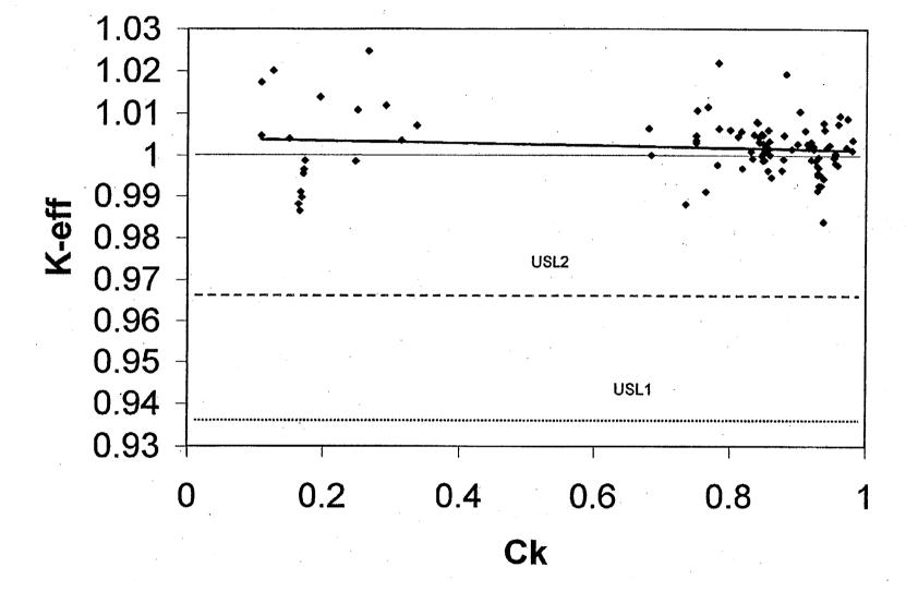
Figure 19 Trend plot for  $k_{eff}$  versus  $c_k$  value for the U(11)O<sub>2</sub> H/X = 500 system
