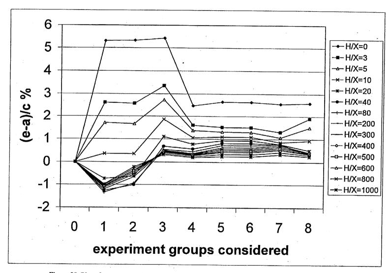
Figure 20 Plot of convergence in predicted  $k_{eff}$  bias, [(e-a)/c], for U(11)O<sub>2</sub> systems as a function of number of experimental groups considered
