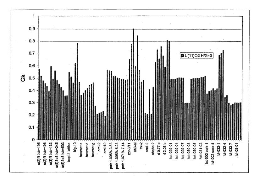
Figure 2 Correlation coefficients,  $c_k$ , for U(11)O<sub>2</sub>, H/X = 3 system with 102 benchmark experiments
