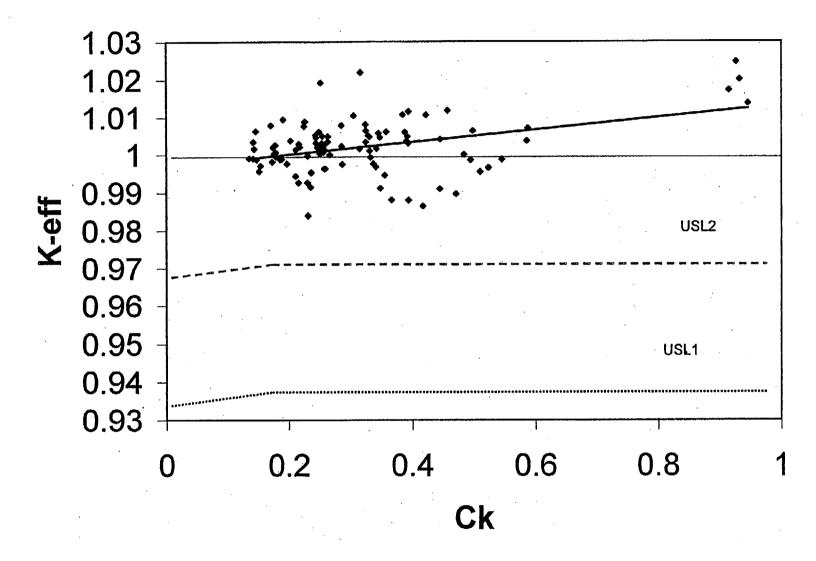
Figure 16 Trend plot for  $k_{eff}$  versus  $c_k$  value for the U(11)O<sub>2</sub> H/X = 0 system
