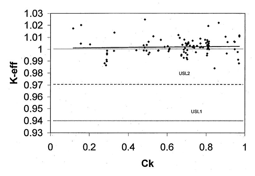
Figure 18 Trend plot for  $k_{eff}$  versus  $c_k$  value for the U(11)O<sub>2</sub> H/X = 40 system
