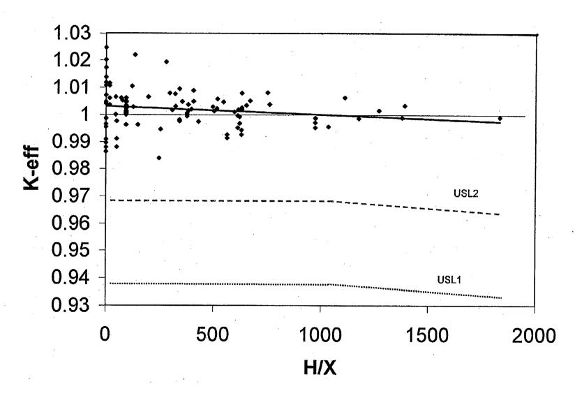
Figure 11 Trend plot for  $k_{eff}$  versus hydrogen-to-<sup>235</sup>U ratio (H/X)
