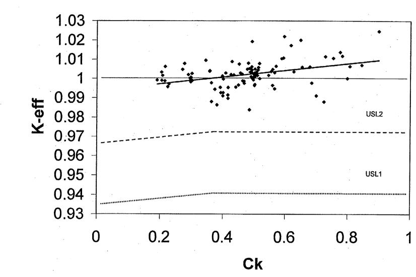
Figure 17 Trend plot for  $k_{eff}$  versus  $c_k$  value for the U(11)O<sub>2</sub> H/X = 3 system
