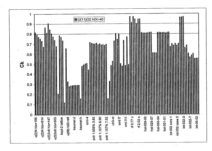
Figure 3 Correlation coefficients,  $c_k$ , for  $U(11)O_2$ , H/X = 40 system with 102 benchmark experiments
