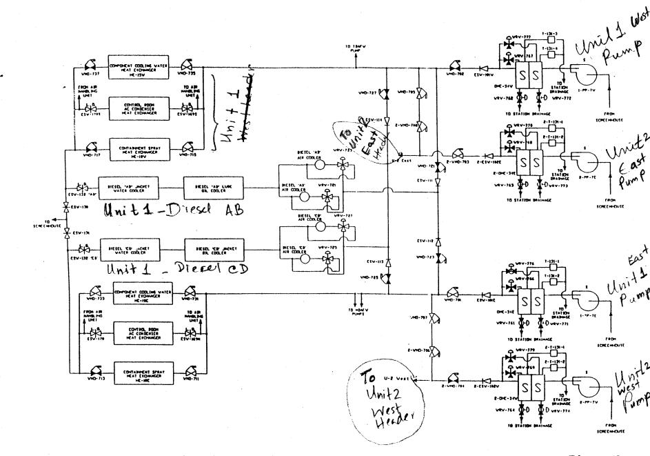
Figure 1 (Issue No. 61): ESW System Simplified Flow Diagram ACTERENCE 344-1405-
