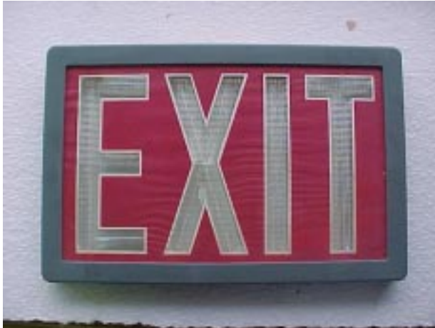
Figure 1 Intact Saunders-Roe Developments Model Betalux-E™ Tritium Exit Sign
