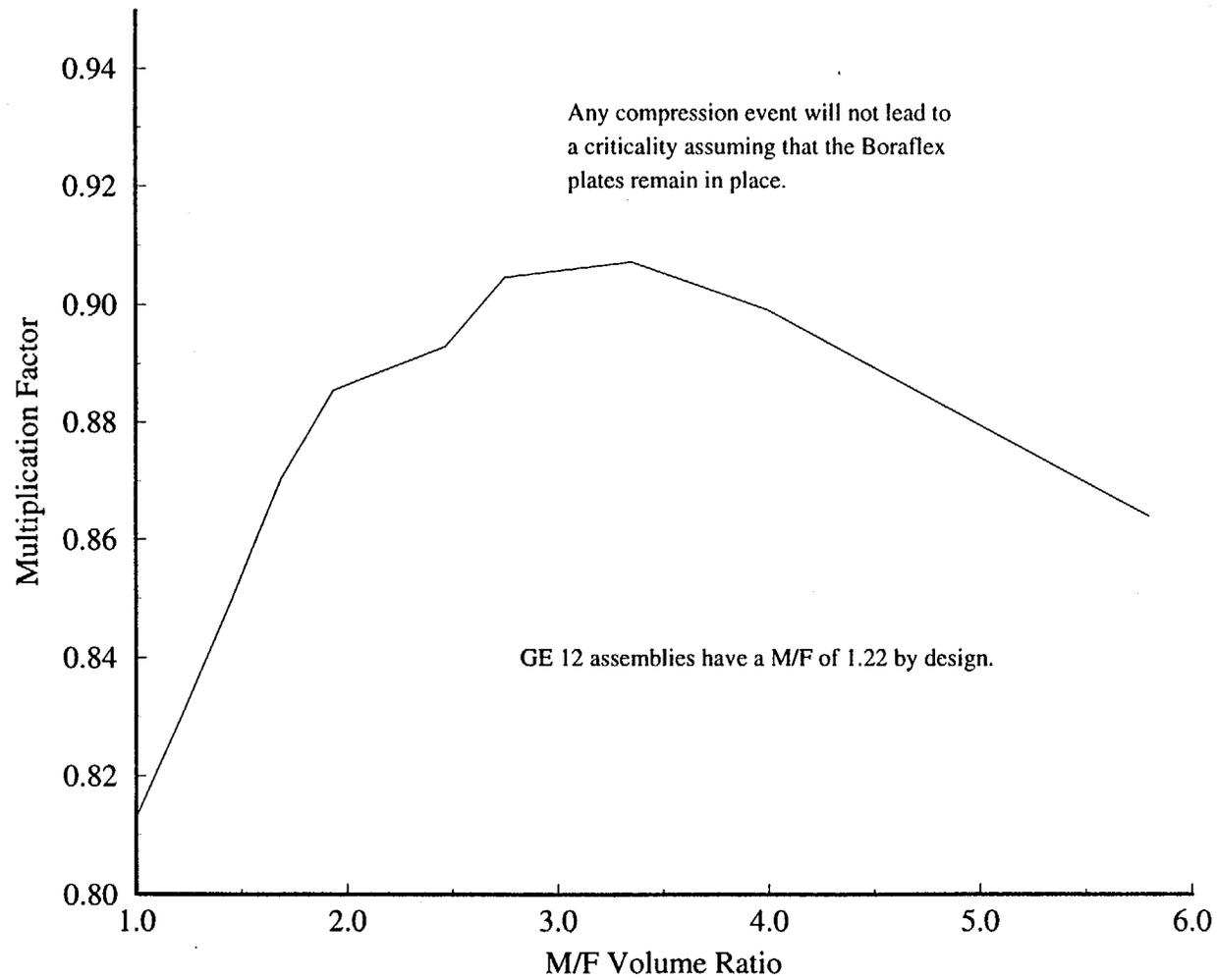
**Figure 4** BWR High Density Storage Rack Eigenvalue following Compressive/Expansion Events
