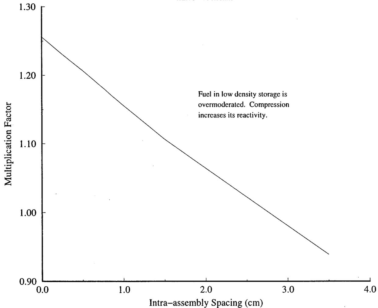
**Figure 2** PWR Low Density Storage Rack Eigenvalue following Compressive/Expansion Events
