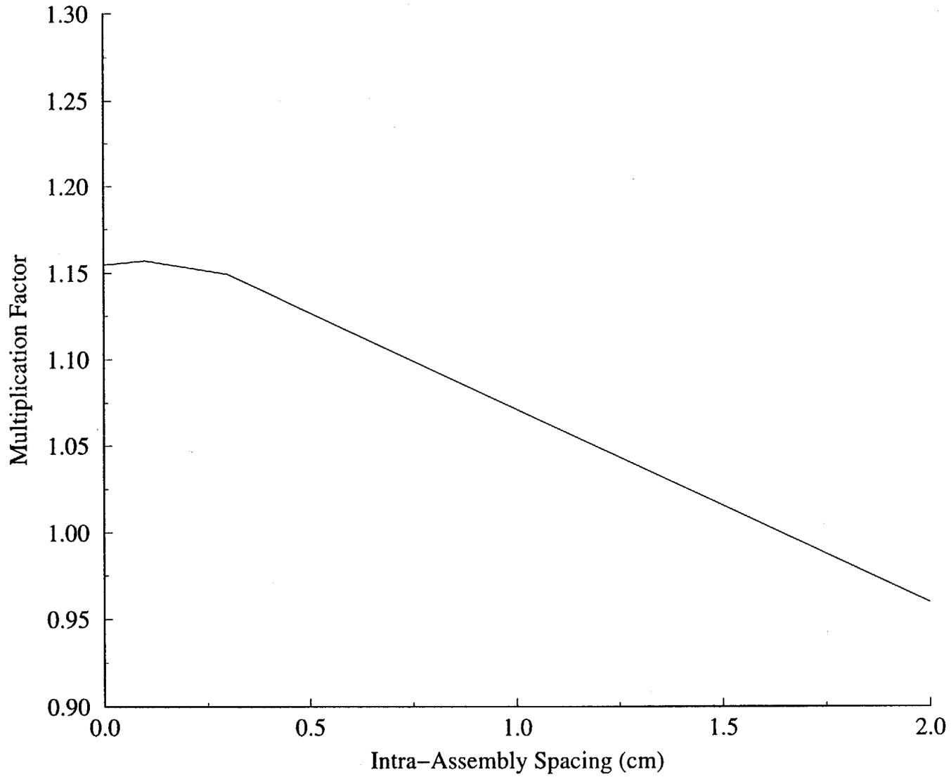
**Figure 5** BWR Low Density Storage Rack Eigenvalue following Compressive/Expansion Events
