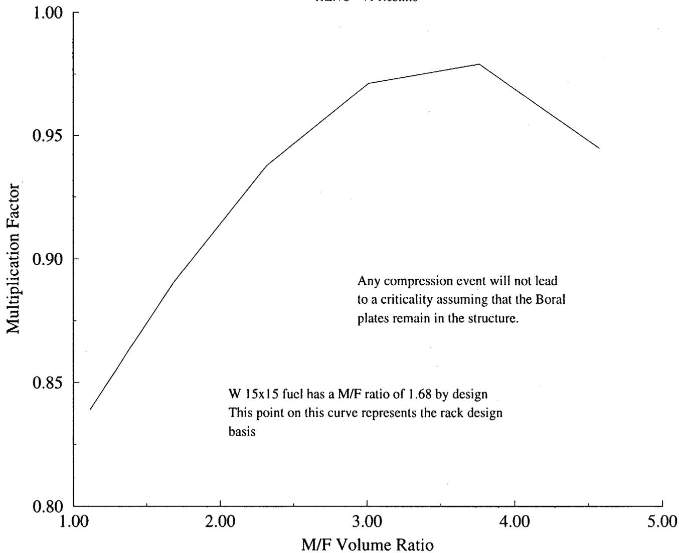
**Figure 1** PWR High Density Storage Rack Eigenvalue following Compressive/Expansion Events
