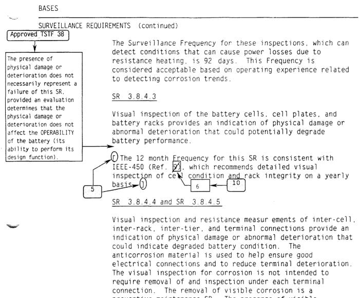
preventive maintenance SR. The presence of visible corrosion does not necessarily represent a failure of this SR provided visible corrosion is removed during performance of SR 3.8.4.4.
