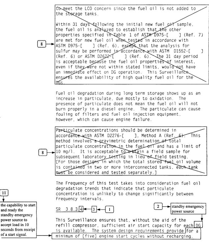
Diesel Fuel Oil - Lube Oil and Starting Air
