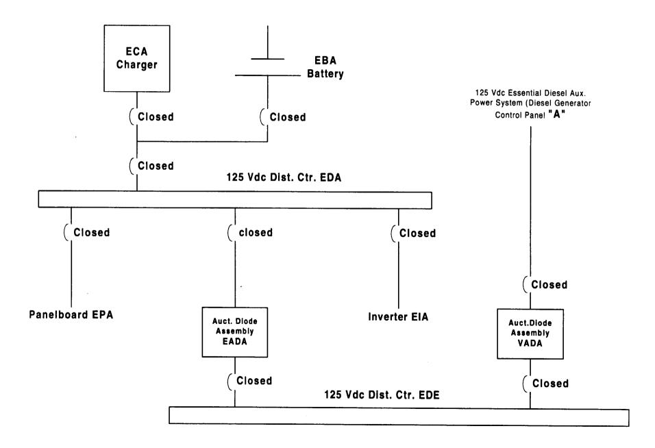
Figure 2: Alignment of Channels A & C During <u>EBA</u> Out of Service
