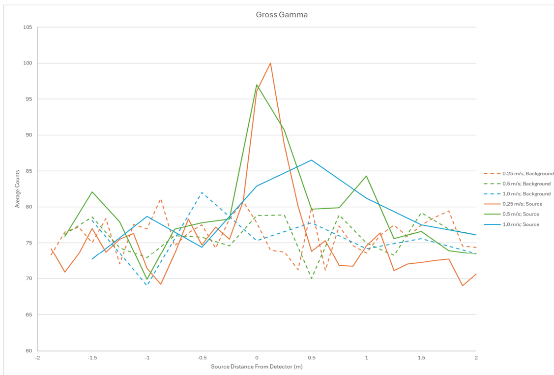
Figure 24 Averaged Benchtop Gross Gamma Background Data and Cs-137 Data for 0.25 m/s, 0.5 m/s and 1 m/s Belt Speeds
