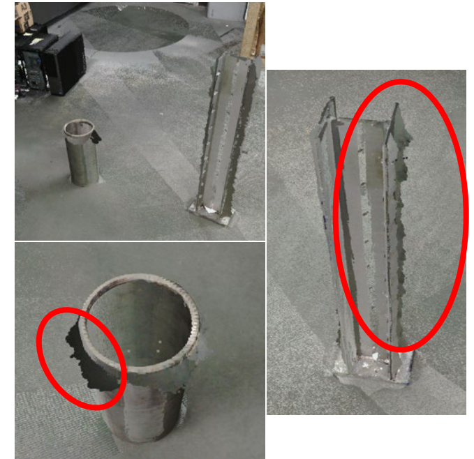
Distortion of Objects with Reflective Surfaces
