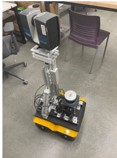
FARO Focus Scanner Mounted onto Jackal Robot
