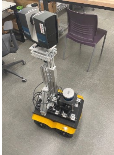
FARO Scanner mounted on Jackal Robot
