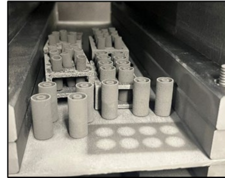
SiC preforms loaded into the BWXT CVI furnace
