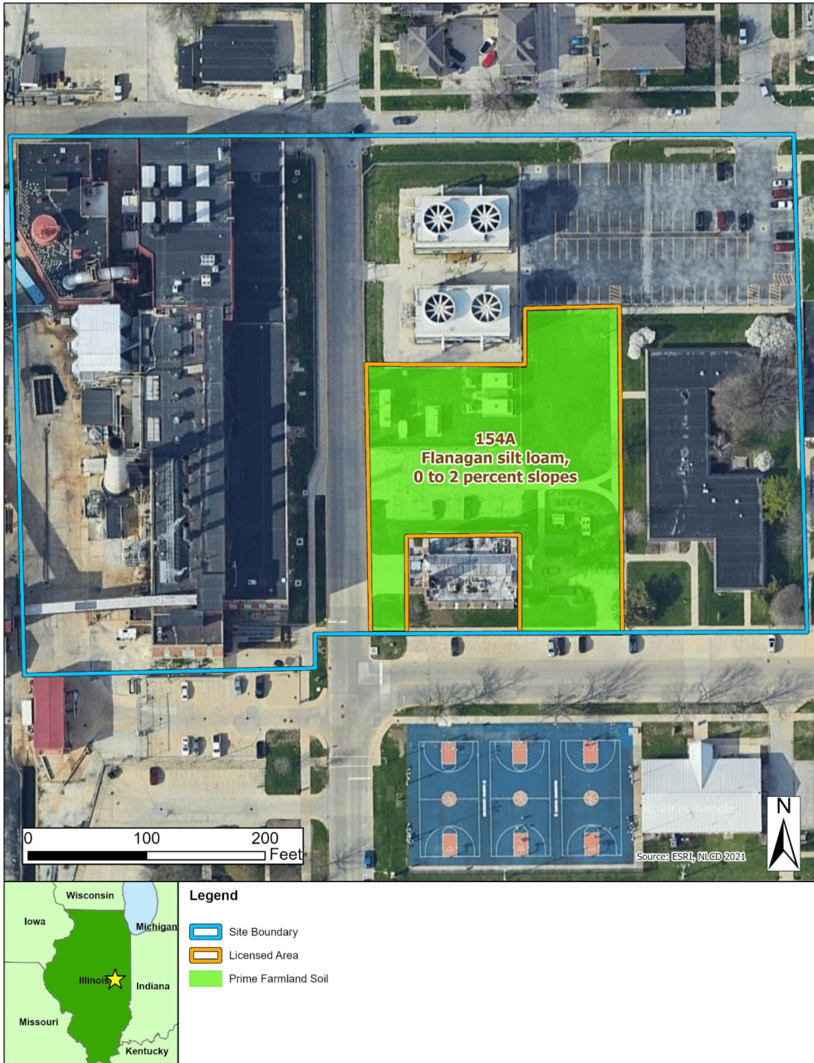
Figure 3-21 NRCS Soil Survey Soil Type Designation at the U. of I. Research Reactor Site
