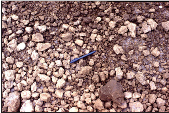
Soil treated with PAM, before rainfall.
