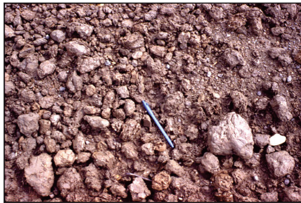
Soil treated with PAM, after rainfall.
