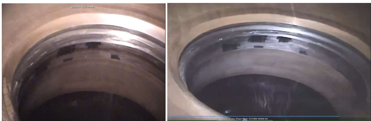
Figure 4-26: CR 2024-1333: SG B Cold Leg Nozzle Blemishes as seen in 2017 (l) and 2024 (r)
