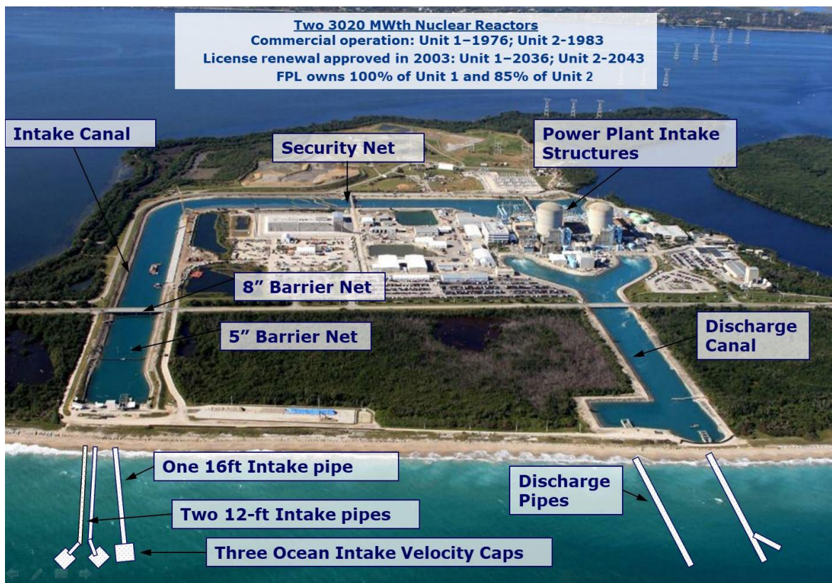
Figure 3-3 Overview of Cooling System at St. Lucie Plant Site. Source: NRC 2019-TN7340.
