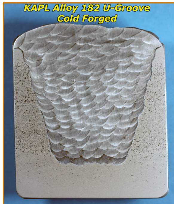
Figure 9. Cross-section optical image of an etched 15% CF KAPL Alloy 182 weld.
