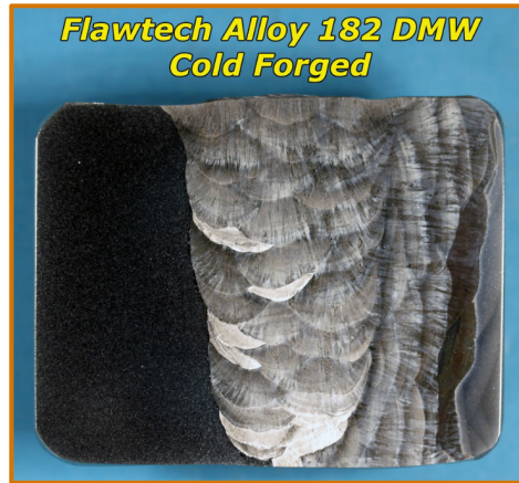
Figure 8. Cross-section optical image of an etched 15% CF Flawtech Alloy 182 weld.
