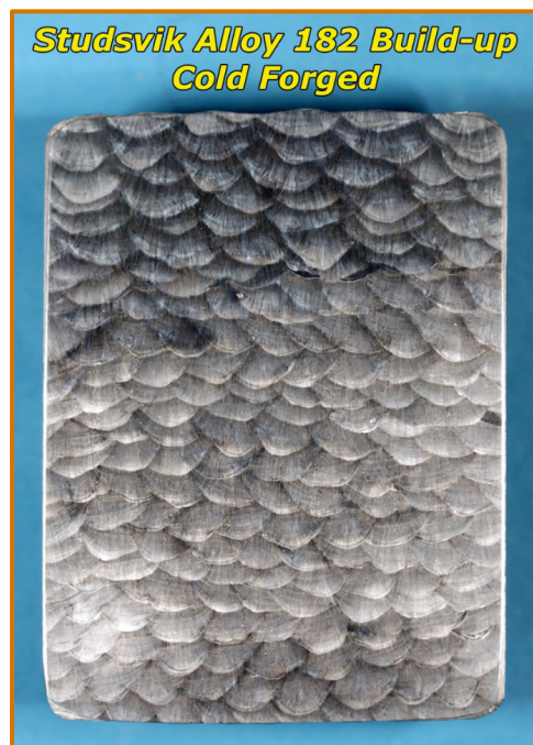
Figure 11. Cross-section optical image of an etched 15% CF Studsvik Alloy 182 weld.
