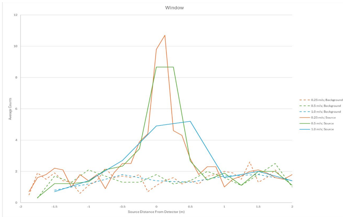
Figure 9-16 Averaged Benchtop Background Data and Cs-137 Data within 662 keV Window for 0.25 m/s, 0.5 m/s and 1 m/s
