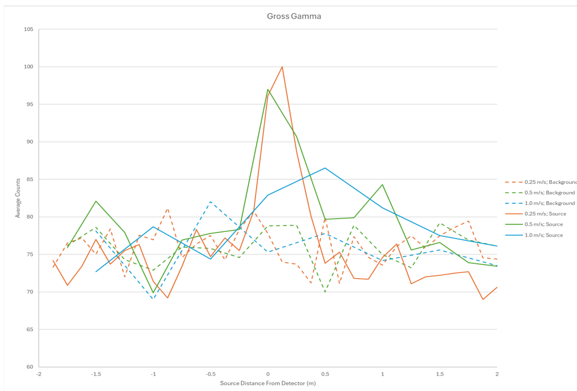
Figure 9-15 Averaged Benchtop Gross Gamma Background Data and Cs-137 Data for 0.25 m/s, 0.5 m/s and 1 m/s
