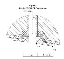
Note: Extent of examination above the original J-groove weld is 1-1/2". The extent of examination on the surface of the new weld covers the ground face of the pad, excluding the blended radius between the new weld and the RVCH cladding.
