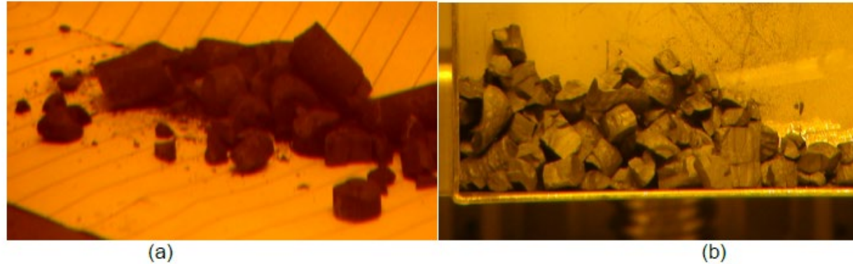
Figure 4-42 Images of fuel particles collected from test rod (a) 196 and (b) 198 revealing large fragments
