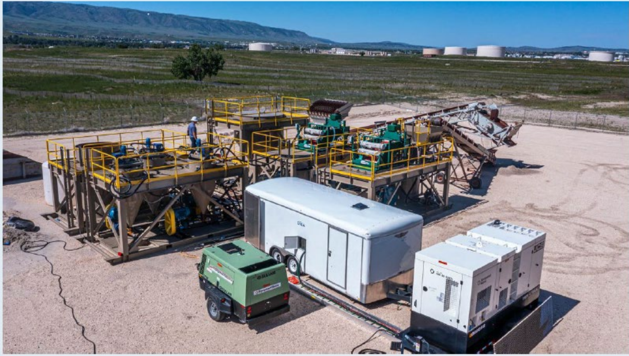
Figure 5. HPSA Unit of 20 Ton/Hour Capacity (DISA 2025b).
