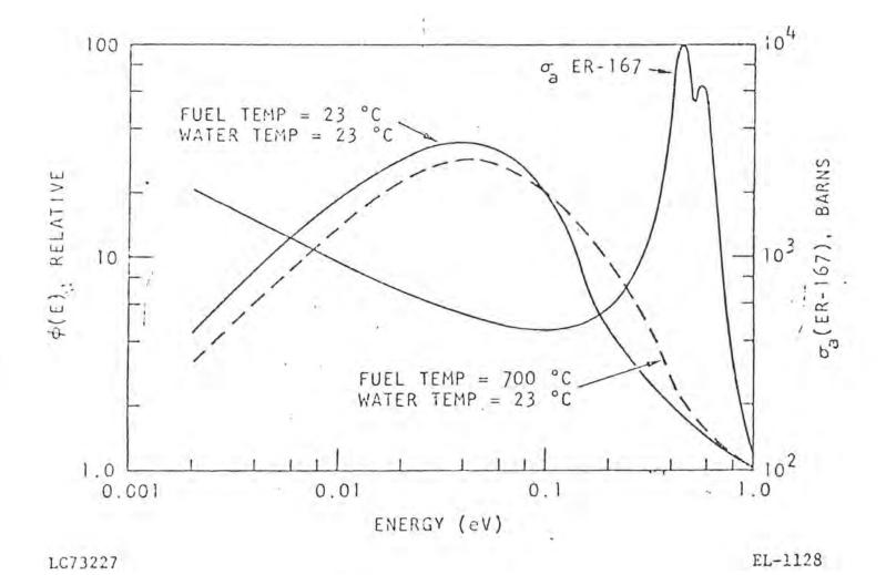
TRICA-FLIP Core--thermal neutron spectra vs fuel temperature relative to  $\sigma_a$  vs energy for Er-167
