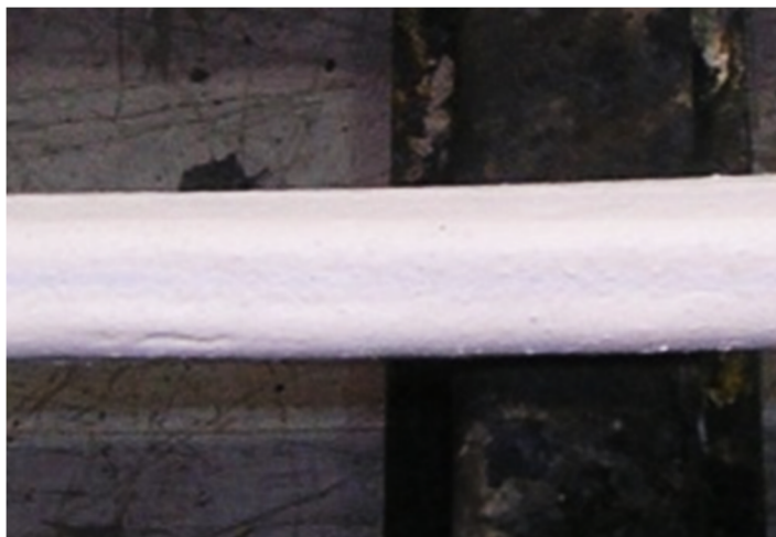
Figure 3-3. Fully cured Vimasco 3i on a cable sample.
