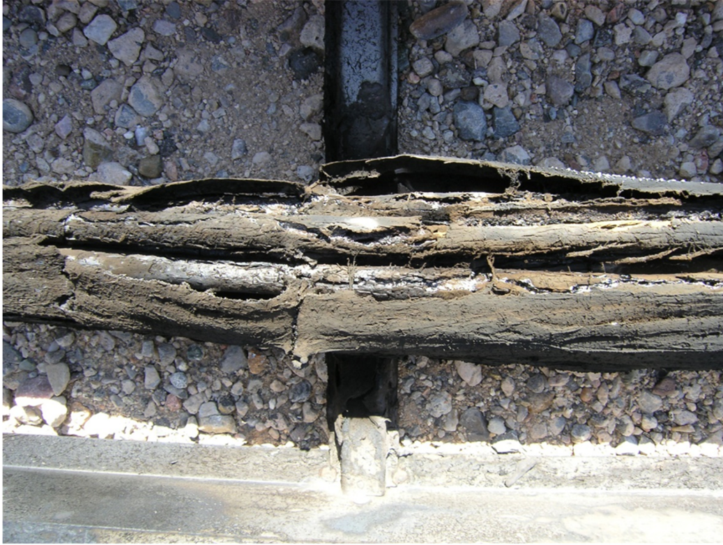
Figure C-16. Closeup photo of separated cable bundle.
