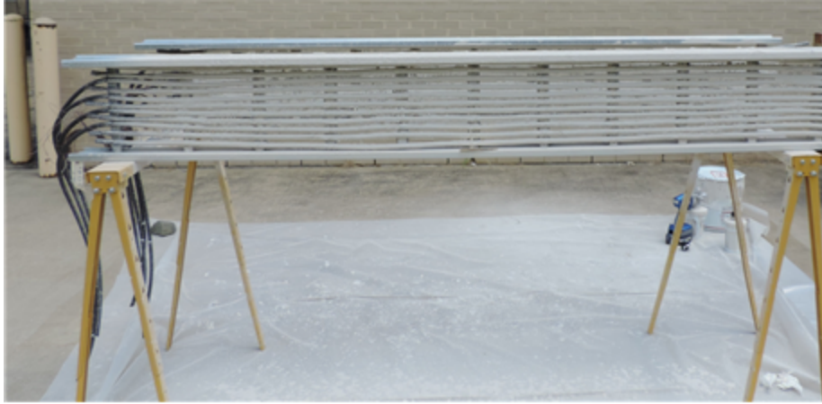
Figure 6-2. Cable tray assembly following application of coating, showing longer cable leads at left for connection to SCDU.
