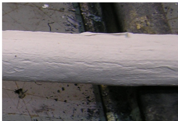
Figure 3-2. Fully cured Flamemastic F-77 on a cable sample.
