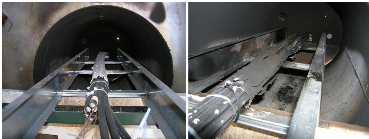
Figure C-15. Before and after photos of the cable bundle separation behavior.
