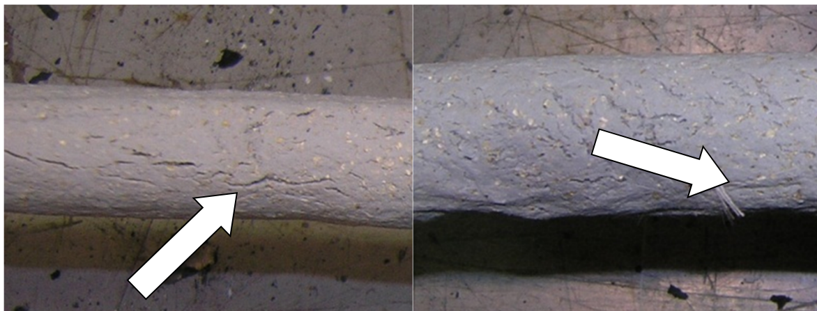
Figure 3-1. Cracking (left) and fibers (right) in the Carboline Intumastic 285 coating along cables.
