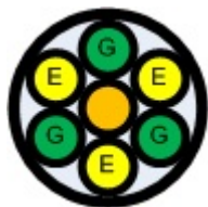
Figure 7-2. Illustration of modified SCDU cable connection (“E” energized conductor; “G” grounded conductor).
