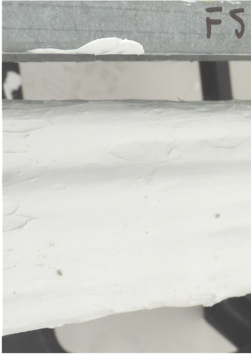
Figure 3-4. Fully cured FS15 on a sample of cables.
