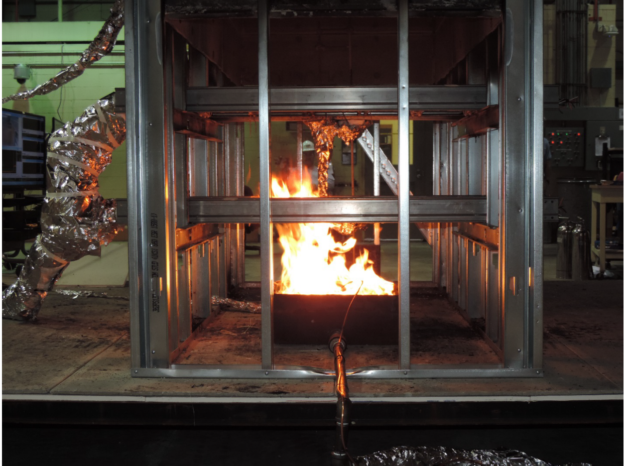
Figure 8-2. End view of the experiment compartment, showing the burner at 50 kW.
