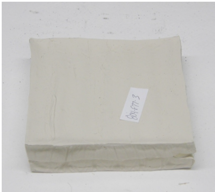
Figure 4-1. Cable segments coated with Flamemastic F-77.
