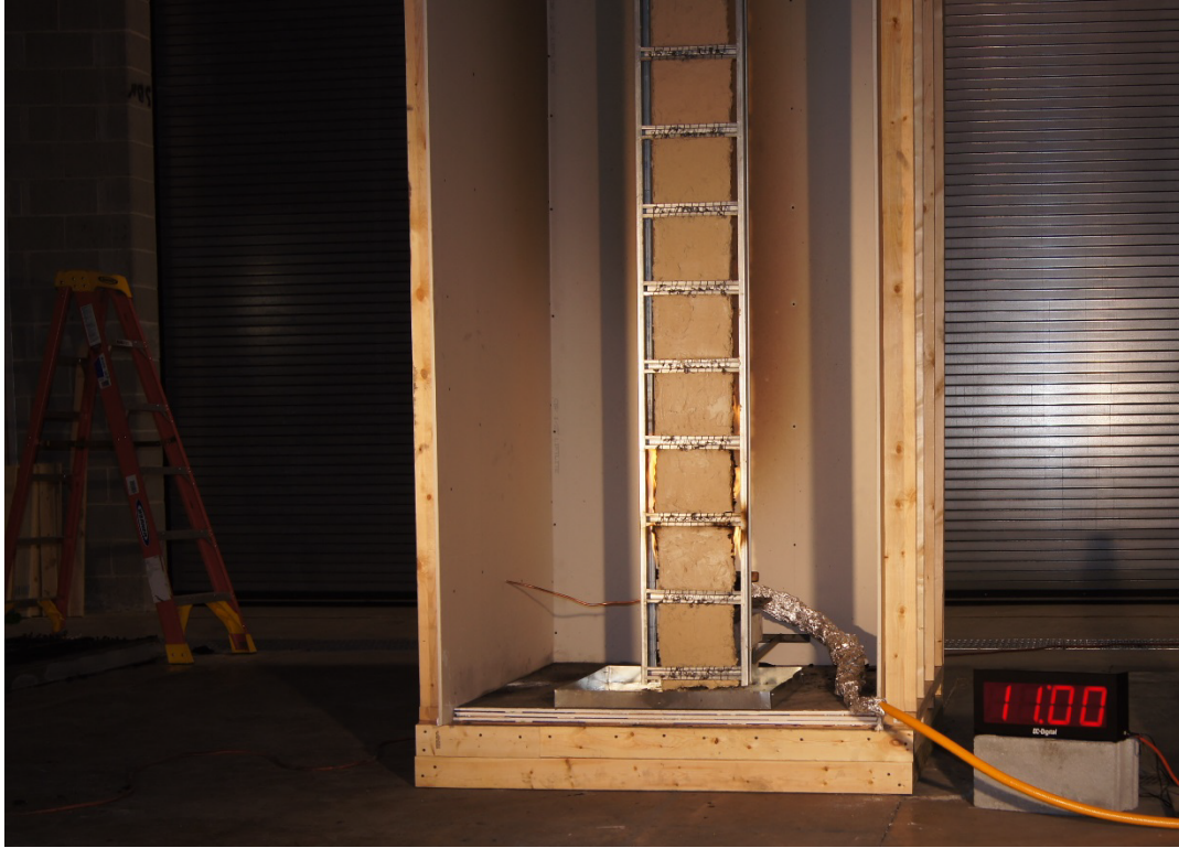
Figure 6-21. Photograph of cable 900 coated with Carboline 285.
