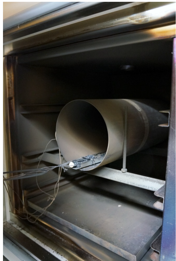
Figure 5-3. Oven interior showing electrodes, gas inlets, thermocouples, shroud, and cable.
