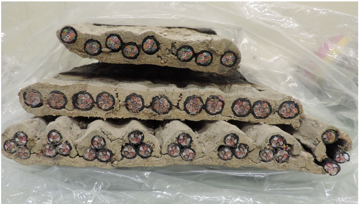
Figure 6-7. Cross-sectional view of the three different cables coated with Carboline.
