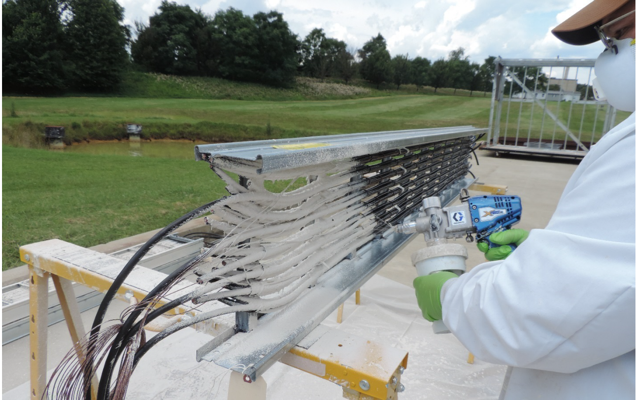
Figure 6-6. Applying the cable coating FS15 via a sprayer.
