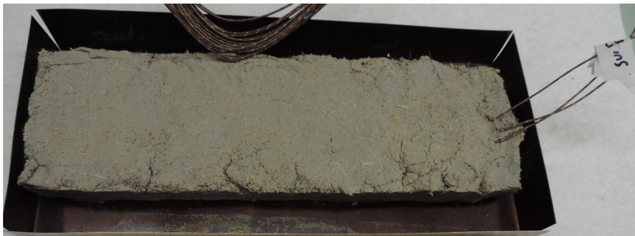
Figure 5-9. Cables coated with Carboline Intumastic 285.
