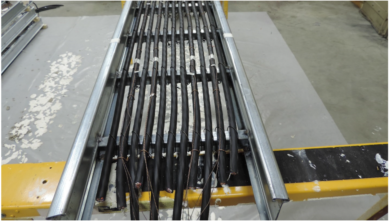
Figure 6-2. Typical configuration of uncoated cables attached to a tray.
