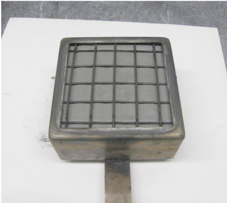
Figure 4-6. Cable 802 coated with Vimasco 3i.
