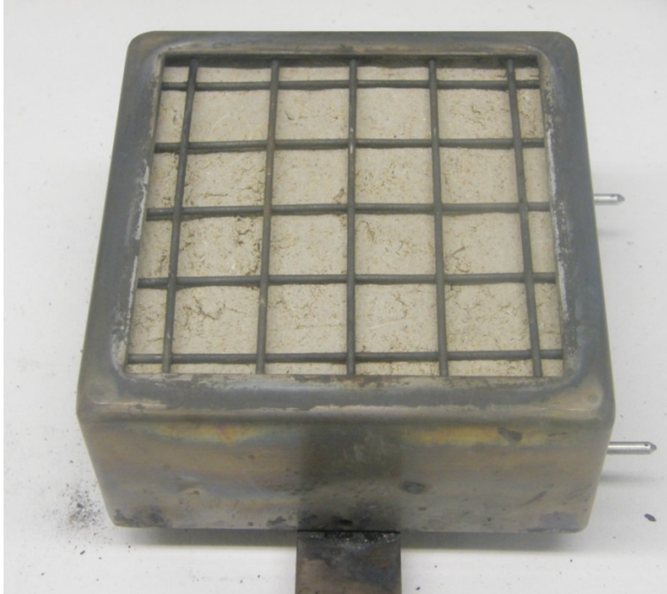
Figure 4-5. Cable 802 coated with Carboline Intumastic 285.
