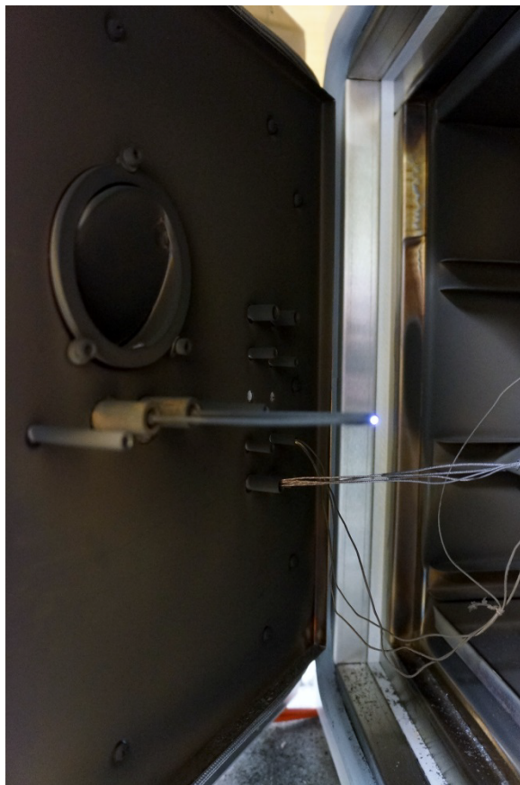
Figure 5-3. Oven interior showing electrodes, gas inlets, thermocouples, shroud, and cable.
