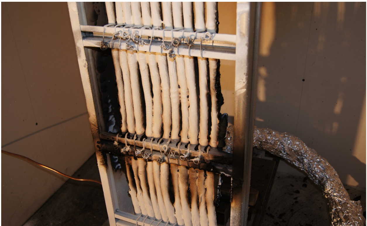
Figure 6-13. Photograph of cable 900 coated with FS15 after experiment I-8.
