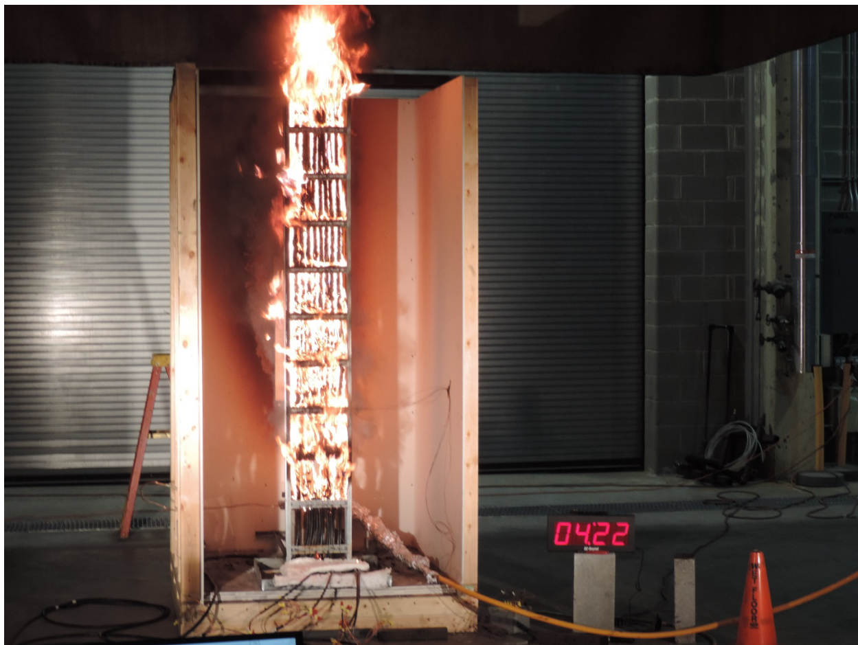
Figure 6-23. Photograph of experiment II-7, cable 902 uncoated.
