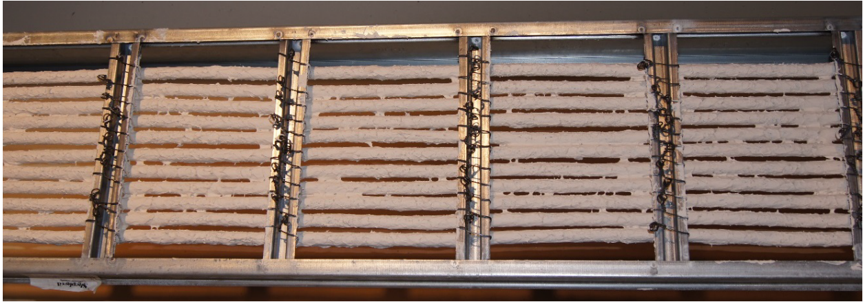
Figure 6-14. Photograph of cable 900 coated with Flamemastic 77.
