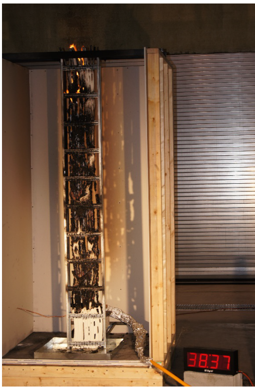
Figure 6-18. Photograph of experiment I-9, cable 900 coated with Vimasco 3i.
