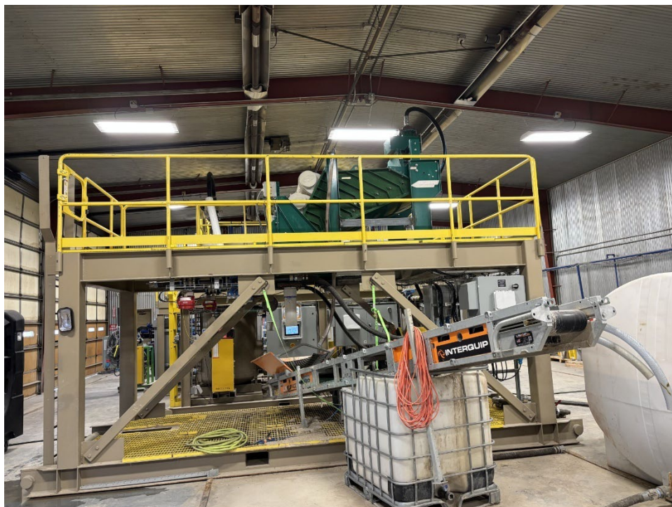
Figure 11-3: 10 TPH Unit Crushing/Grinding Skid
