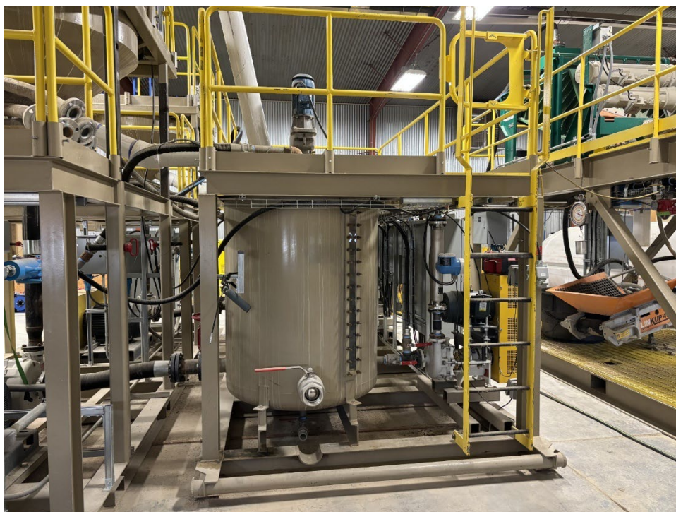
Figure 11-2: 10 TPH Unit Mixing Skid
