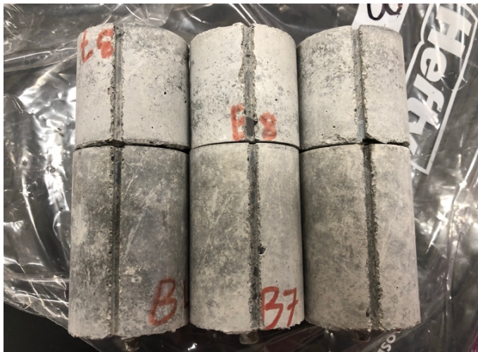
Figure 3-6 Irradiation Testing Specimens Cut to Create a 2 × 2 mm Groove for Placement of the TC at Mid-Height of the Specimen Stack
