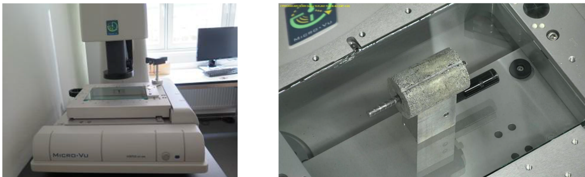
Figure 5-1 (Left) Vertex Touch Probe Measurement Device; (Right) Pullout Specimen Setup for Height Measurement
