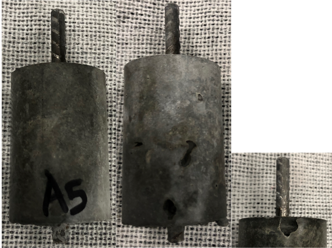
Figure 3-4 (Left) Specimen A05R (Concrete Con-A) Showing a Few Small Surface Pores, (Center) Specimen A06R Showing Larger Surface Defects, and (Right) Specimen A11R Showing a Large Defect Near the Top Surface
