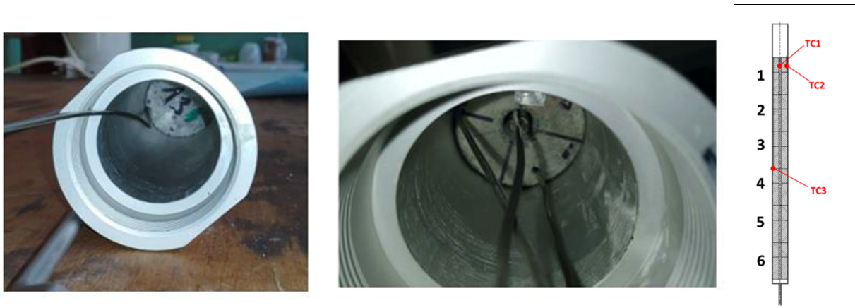
Figure 2-11 (Left) View of the Thermocouple (TC) Placed at the Capsule Mid-Height, (Center) View of the Two TCs Installed in the Top Specimen, and (Right) Drawing Showing the TC Locations
