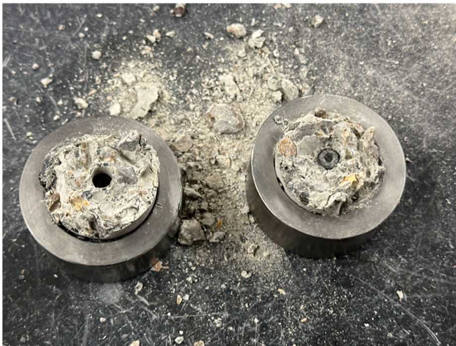
Figure 5-10 Post Compression Test Showing the Fractured Surface of the Concrete Specimen
