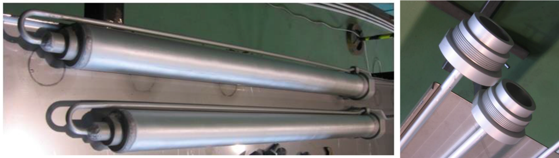
Figure 2-5 Photographs of the Capsules (Left) and Upper Plugs (Right) Fabricated at CVR
