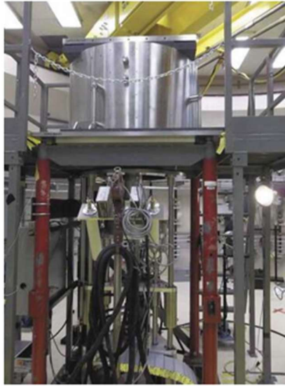
Figure 5. Photo of KRUSTY on the Comet machine
