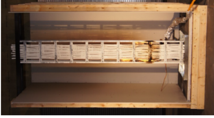
Photograph of experiment I-8, cable 900 coated with FS15.
