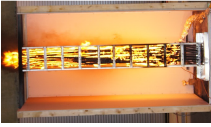
Photograph of experiment I-4, cable 900, uncoated.
