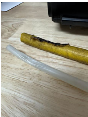
inner white sleeve melted into cable inside of yellow guide. .jpg
