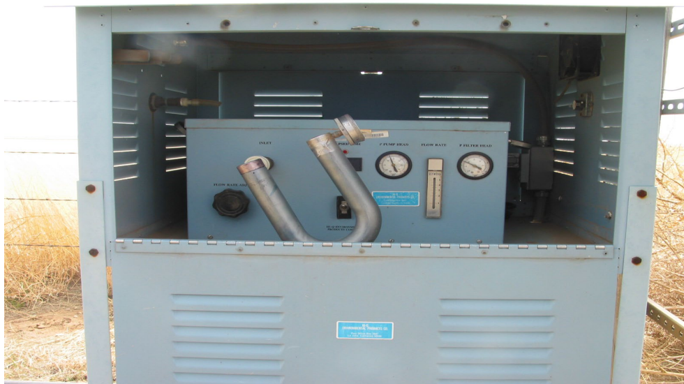
Fig. 5.4. Low-volume sampling apparatus.
