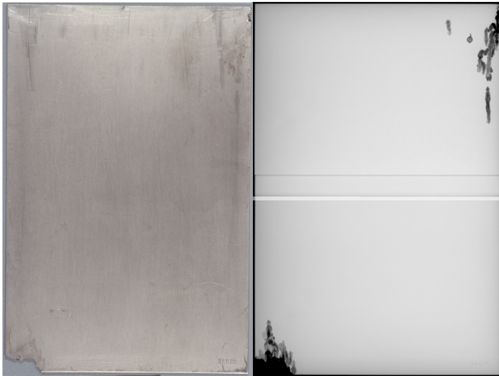
FIGURE 18. Type 304 SS sensitized (front of 56D20 ). Cleaned specimen (left) and X-ray (right).
