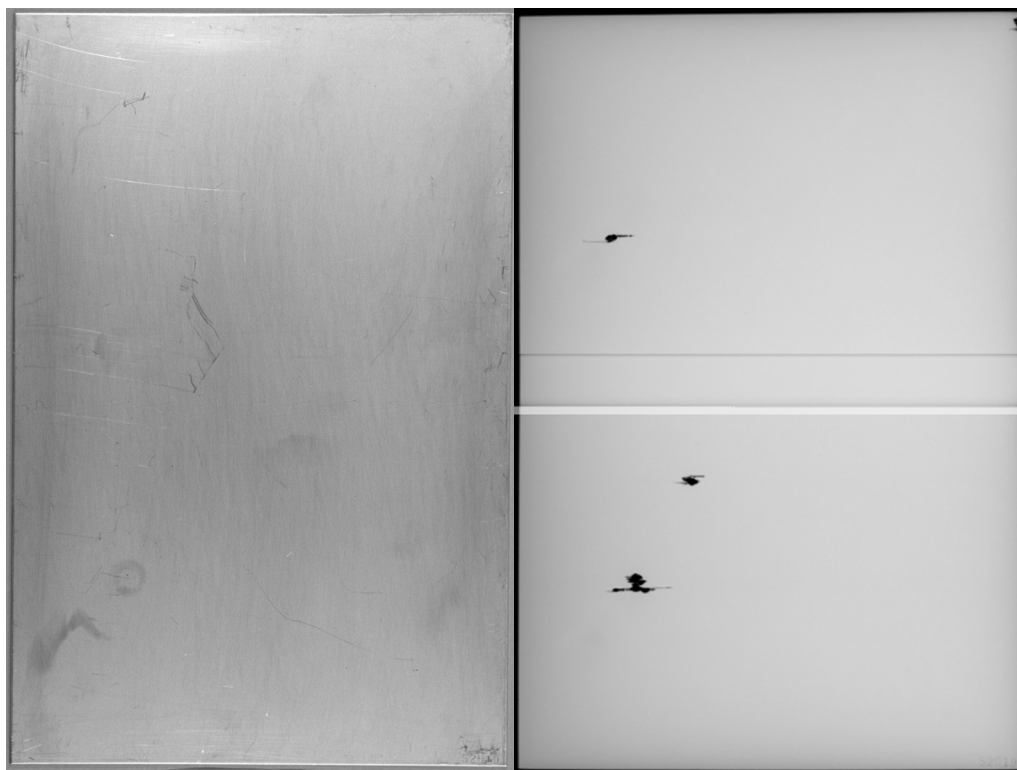
FIGURE 1. Type 301 SS annealed (front of 52D19). Cleaned specimen (left) and X-ray (right).
