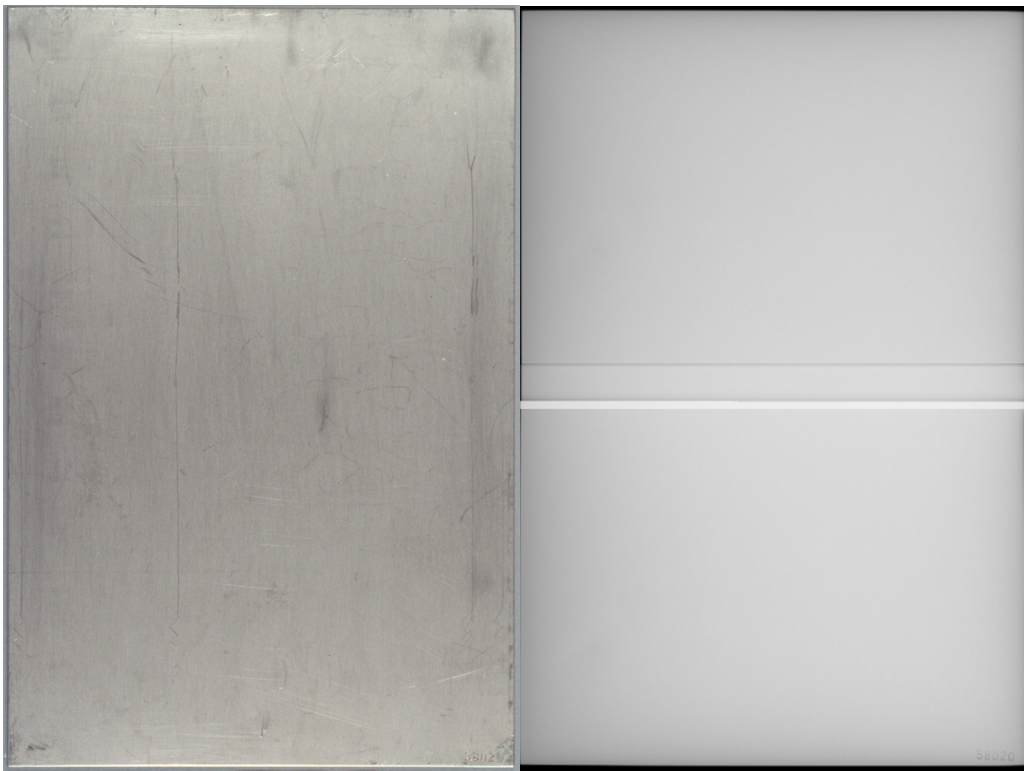
FIGURE 22. Type 316 SS annealed (front of 58D20). Cleaned specimen (left) and X-ray (right).
