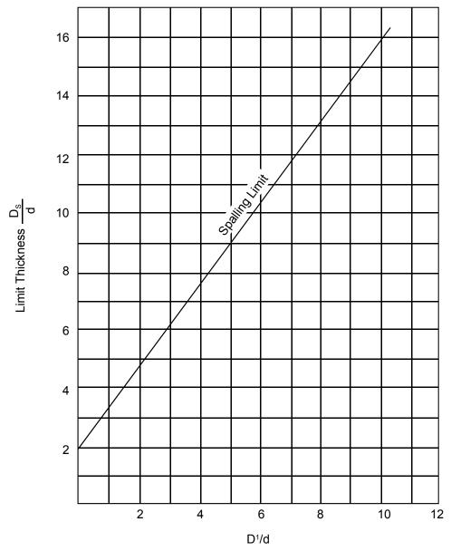
$D^1$  = Penetration d = Diameter of Missle  $D_S$  = Thickness required to Prevent Spalling
