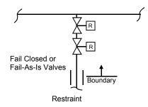
Note: The Reactor Coolant Pump No. 1 Seal Is Assumed To Be Equivalent To First Valve
