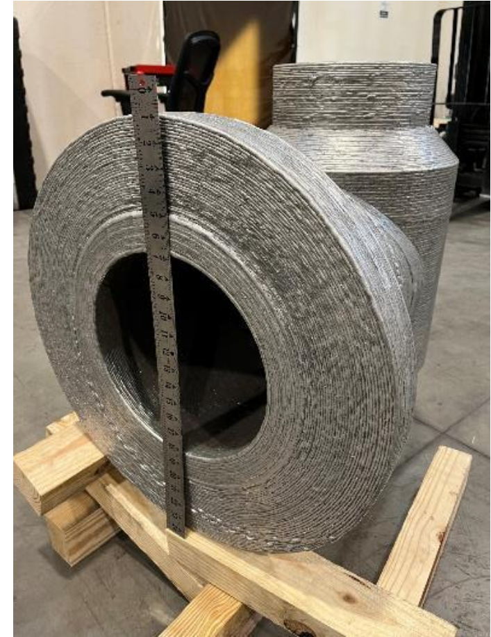
316LSi valve body, 1600 pounds (700 kg) Collaborative effort between EPRI and Lincoln Electric Additive Solutions
