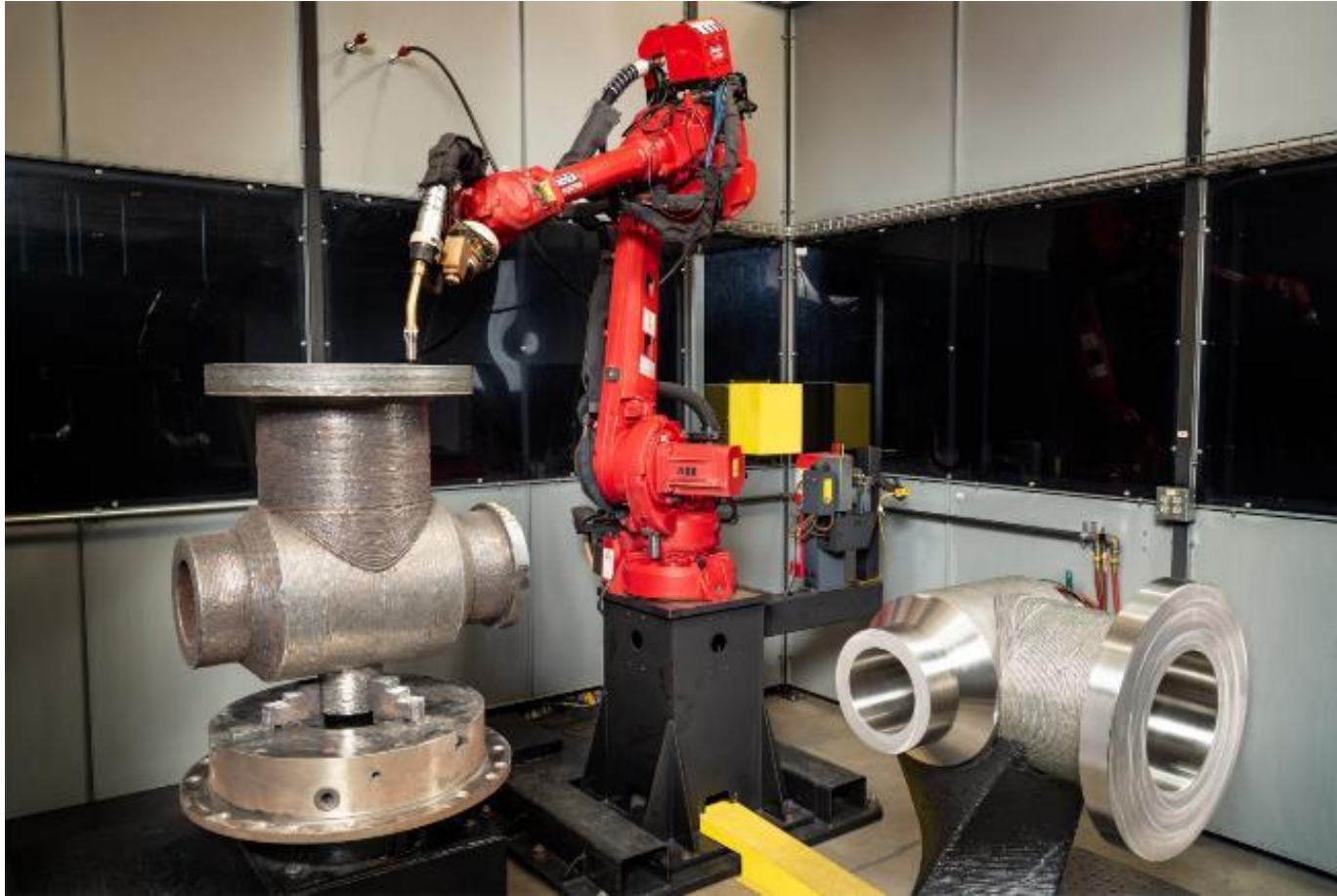
316LSi valve body, 1600 pounds (700 kg) Collaborative effort between EPRI and Lincoln Electric Additive Solutions
